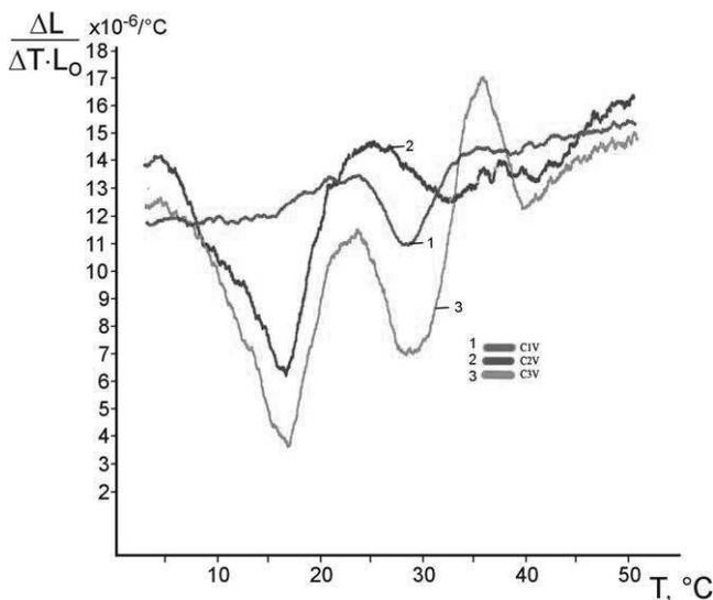
Fig. 3. First differential curves  $(\Delta L/\Delta T)/L_0=f(T)$  of the model alloys containing 0.31-1.25% C, about 0.4% V and strong background of the other alloying elements
