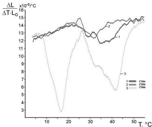
Fig. 2. First differential curves  $(\Delta L/\Delta T)/L_0=f(T)$  of the model alloys containing 0.17-0.59% C, about 2% Mn and weak background of the other alloying elements
