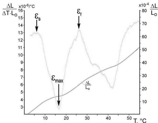
Fig. 1. Example of the dilatogram  $\Delta L/L_0=f(T)$  recorded during heating up step ( $V=0.5^\circ\text{C/s}$ ) of a tempered specimen made of the C3<sub>Mn</sub> model alloy (0.59% C, 2% Mn), first differential curve  $(\Delta L/\Delta T)/L_0=f(T)$  and method of determination of the  $\epsilon_s$ ,  $\epsilon_f$ ,  $\epsilon_{max}$  temperatures
