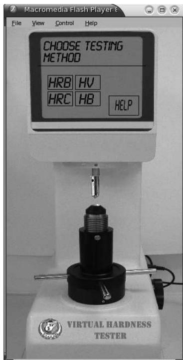
Fig. 3. Virtual simulation of hardness tester, presented is the panel serving for the choice of the testing method
