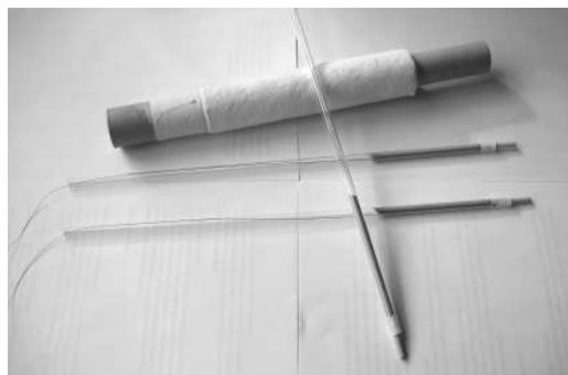
Fig. 1. Measuring probe TSO 6 and sensors for continuous measurement of oxygen activity
