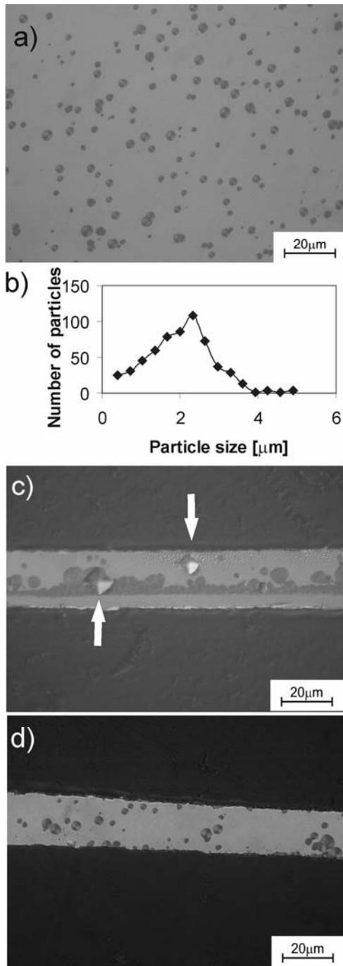
Fig. 2. The typical microstructure of the melt spun ribbon; a) longitudinal section, b) particle size distribution of the spherulitic grains, c) cross-section, d) massive colonies of spherulitic grains in the amorphous matrix with Vickers indenter traces
