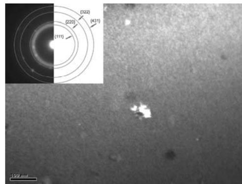
Fig. 3. TEM microstructure with diffraction pattern. Ag-rich particles included in amorphous matrix
