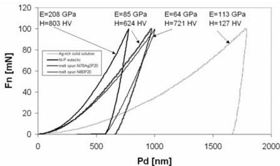
Fig. 4. Indentation curves with Young modulus and hardness results for Ag-rich crystalline solid solution, Ni-P base crystalline matrix, melt spun  $\text{Ni}_{80}\text{P}_{20}$  amorphous alloy, melt spun  $\text{Ni}_{78}\text{Ag}_2\text{P}_{20}$  amorphous/crystalline composite
