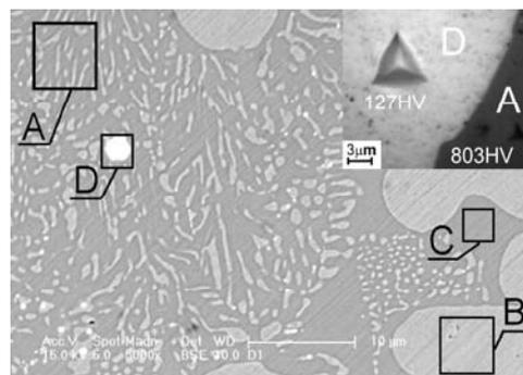
Fig. 1. SEM primary microstructure of the arc melted droplet; exemplary EDS analysis for the structure constituents: A – 80.06at.% Ni, 19.94at.% P; B – 98.16at.% Ni, 1.84at.% P; C – 74.29at.% Ni, 25.71at.% P; D – 96.52at.% Ag, 3.48at.% Ni; micro-hardness indentations in the Ni-P-rich and Ag-rich regions
