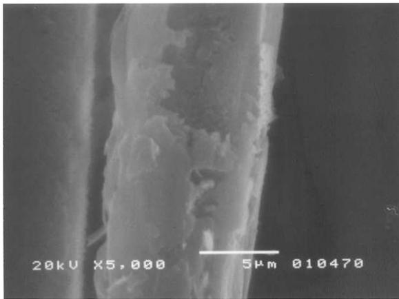
Fig. 3. A damaged area in PBO fiber sample from high discharge voltage
