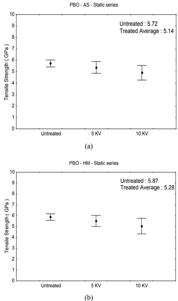
Fig. 4. The effects of electrostatic discharge treatment on the tensile strength of (a) AS and (b) HM PBO fibers
