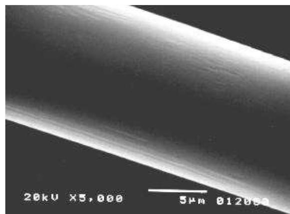
Fig. 1. SEM micrograph of the untreated AS PBO (AS-UT) fiber sample
