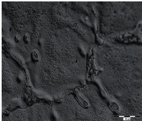
Fig. 4. Alloys AZ91, AZ61, AZ31 without heat treatment, after torsion test (Nomarski contrast)
