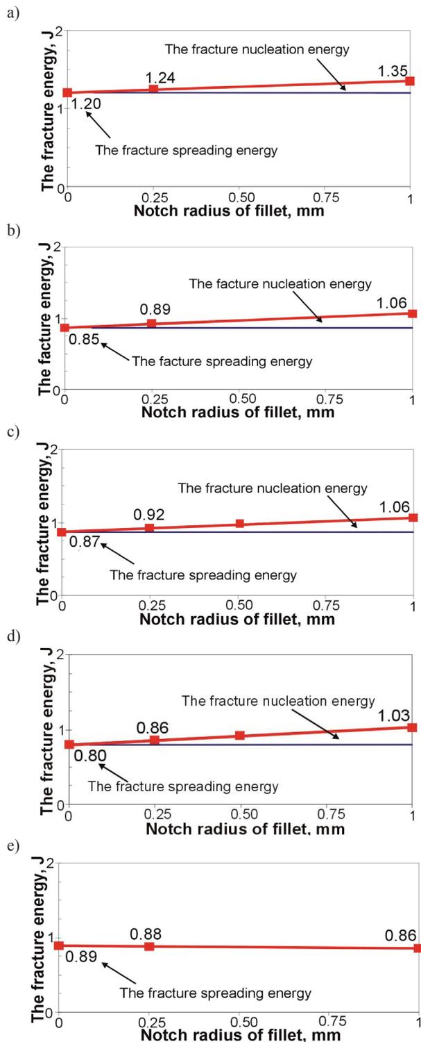
Fig. 7. Method of defining fracture spread work on the basis of the work of breaking KCU2 and KCV using Gulajev's interpretation [15]: (a) delivery condition, (b) cooling at 200°C/h, (c) cooling at 48°C/h, (d) cooling at 30°C/h, (e) cooling at 12°C/h
