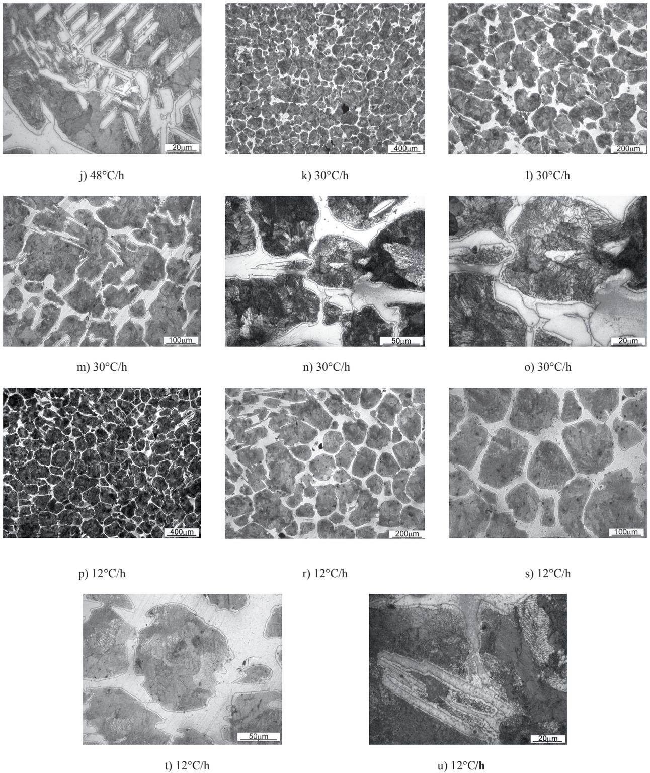
Fig. 3. Structures of G200CrMoNi4-6-3 cast steels heated to 1150°C and cooled at various rates: (a – e) cooling at 200°C/h, (f – j) cooling at 48°C/h, (k – o) cooling at 30°C/h, (p – u) cooling at 12°C/h
