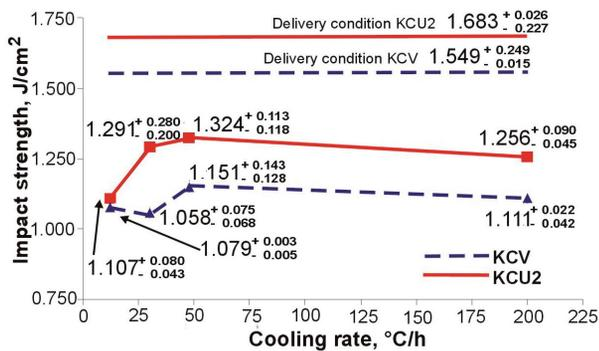
Fig. 4. The effect of cooling rates upon heat treatment on the impact strength of G200CrMoNi4-6-3 cast steel
