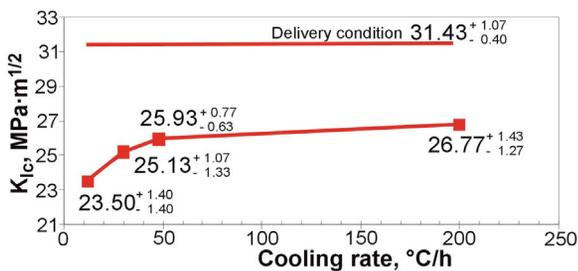
Fig. 5. Effect of cooling rate (upon heat treatment) on  $K_{Ic}$  factor
