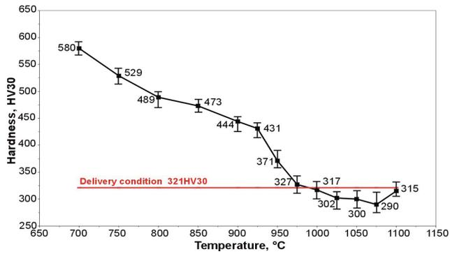
Fig. 2. The effect of austenitizing temperature at hardness samples G200CrMoNi4-6-3 cast steel quenched in oil
