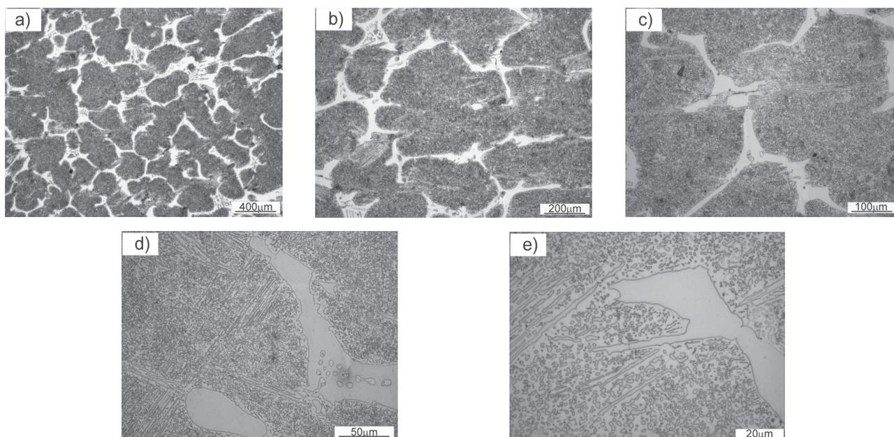
Fig. 1. Microstructure of G200CrMoNi4-6-3 of investigated cast steel (as-delivered condition)
