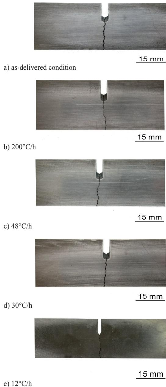
Fig. 6. Picture of fracture after  $K_{Ic}$  test: (a) as-delivered condition, (b) after heat treatment (cooling at  $200^\circ\text{C/h}$ ), (c) after heat treatment (cooling at  $48^\circ\text{C/h}$ ), (d) after heat treatment (cooling at  $30^\circ\text{C/h}$ ), (e) after heat treatment (cooling at  $12^\circ\text{C/h}$ )
