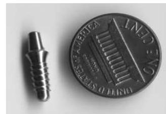
Fig. 6. Manufactured mono-block tooth implant
