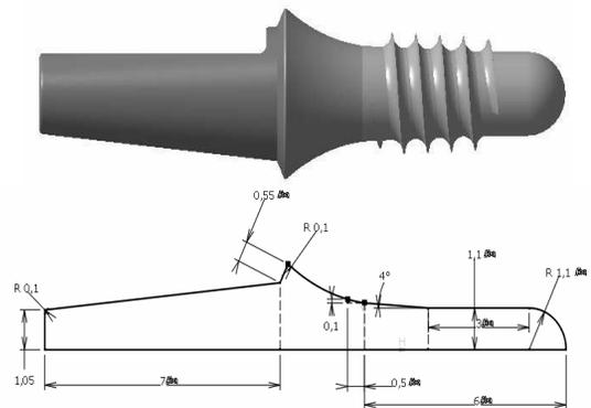
Fig. 3. Function definition for the geometric features
