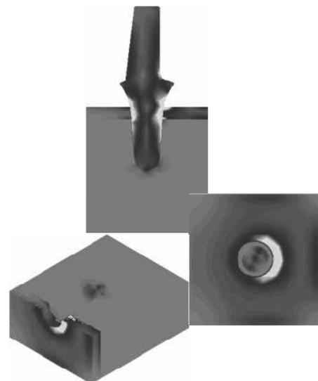
Fig. 9. FEM analysis of the new mono-block implant
