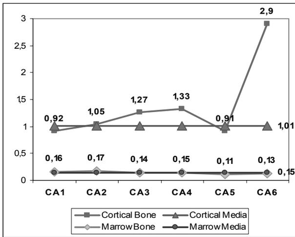
Fig. 10. Results of the FEM Analysis to the dental implant
