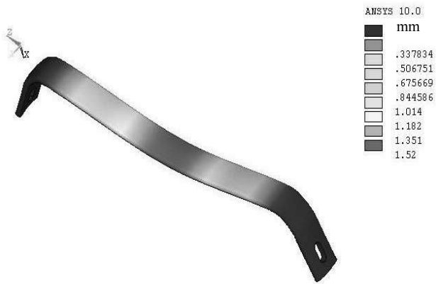
Fig . 4. Displacements distribution in the plate made of stainless steel Cr-Ni-Mo (l= 160 mm and g=2,5 mm)
