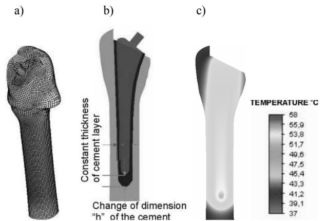
Fig. 1. FEM model of the bone-cement-stem system with a finite elements lattice – (a), its cross-section with shown components – (b) and an example of temperature distribution – (c)
