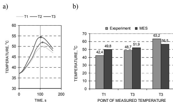
Fig. 5. Temperature dependence on the surgical cement polymerization time determined in a numerical model - (a); a comparison of maximum temperatures determined experimentally and calculated - (b)
