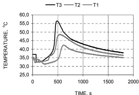
Fig. 4. Dependence of temperature on surgical cement polymerization time in the laboratory model
