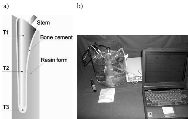
Fig. 2. Lateral cross-section of the laboratory model - (a) and test stand for measuring the surgical cements' polymerization temperature - (b)
