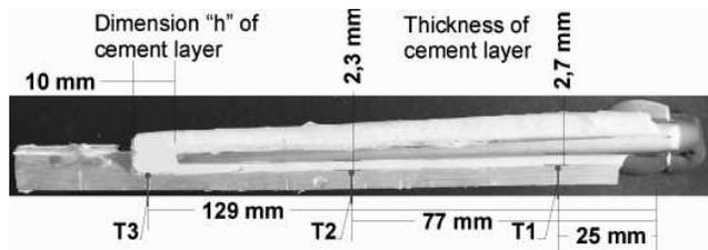
Fig. 3. Method of thermocouples arrangement in the laboratory model
