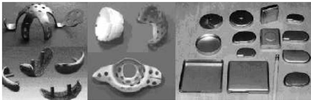
Fig. 1. Some examples of the titanium products made by stamping technology [12, prospectus]
