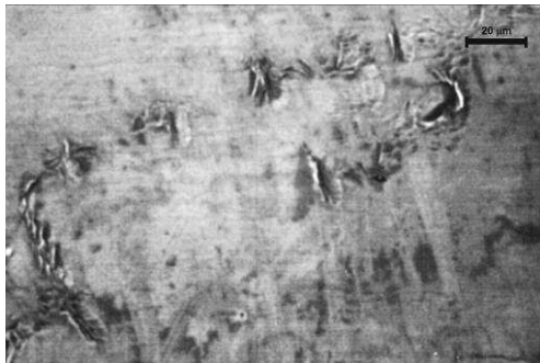
Fig. 7. Locally etched areas on the passivated surface of the electrodes (cathode) after 24 weeks of electrostimulation, SEM
