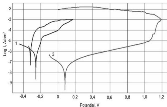
Fig. 2. Anodic polarization curves of samples made of X39Cr13 steel: 1 – barrel finishing with DLC coating (magnetron method), 2 – barrel finishing, passivation with DLC coating (magnetron method)
