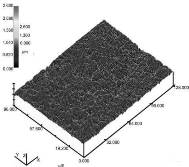
Fig. 3. Topography of the surface barrel finishing, passivation with DLC coating of samples by means of the magnetron methods
