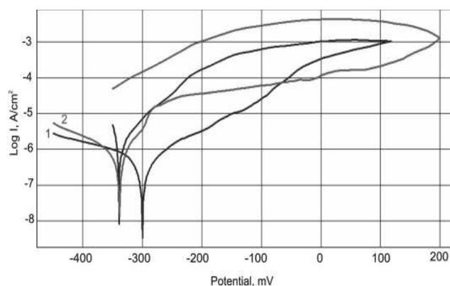
Fig. 1. Anodic polarization curves of samples made of X39Cr13 steel: 1 - barrel finishing with DLC coating (RF PACVD method), 2 - barrel finishing, passivation with DLC coating (RF PACVD method)
