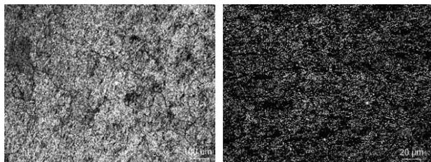
Figs. 5 and 6: Fig. 5. The normal region (in near of the seam line)  $T_B=450^\circ C$ ,  $V_R=15\text{mm/s}$ ,  $T_E=475^\circ C$ ; Fig. 6. The normal reion (no-weld)  $T_B=450^\circ C$ ,  $V_R=15\text{mm/s}$ ,  $T_E=475^\circ C$
