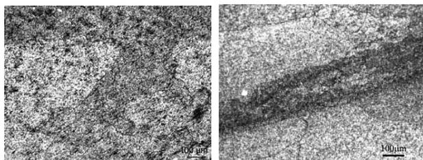
Figs. 3 and 4: Fig. 3. The microstructure of normal zone  $T_B=430^\circ C$ ,  $V_R=10\text{mm/s}$ ,  $T_E=440^\circ C$ ; Fig. 4. Seam weld region  $T_B=450^\circ C$ ,  $V_R=15\text{mm/s}$ ,  $T_E=475^\circ C$
