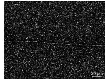
Fig. 2. Seam weld region (in dark)  $T_B=430^\circ\text{C}$ ,  $V_R=10\text{mm/s}$ ,  $T_E=440^\circ\text{C}$
