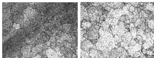
Figs. 9 and 10: Fig. 9. Seam weld region  $T_B=510^\circ C$ ,  $V_R=6\text{mm/s}$ ,  $T_E=560^\circ C$ ; Fig. 10. The normal region (in near of the seam line)  $T_B=510^\circ C$ ,  $V_R=6\text{mm/s}$ ,  $T_E=560^\circ C$
