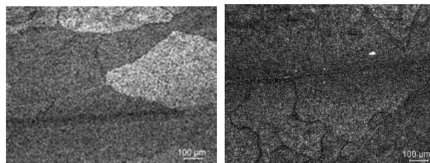
Figs. 7 and 8: Fig. 7. Seam weld region  $T_B=470^\circ C$ ,  $V_R=15\text{mm/s}$ ,  $T_E=500^\circ C$ ; Fig. 8. Seam weld region  $T_B=490^\circ C$ ,  $V_R=15\text{mm/s}$ ,  $T_E=520^\circ C$
