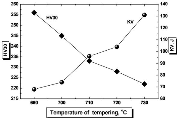
Fig. 7. Influence of tempering temperature on changes of hardness and impact energy
