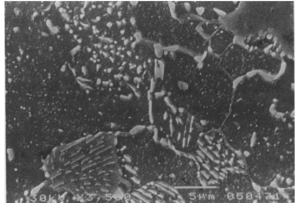
Fig. 2. Structure of the investigated cast steel after service
