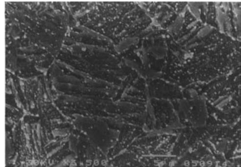
Fig. 6. Structure of the cast steel after regenerative heat treatment
