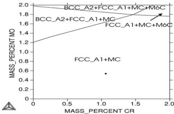
Fig. 4. Isothermal section of investigated cast steel calculated using THERMO – CALC at 1180K, position of the cast steel is marked by solid circle
