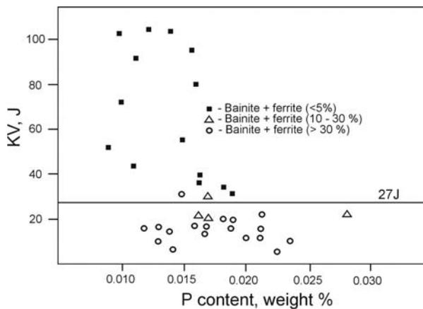
Fig. 1. Influence of the phosphorus content and microstructure on the impact energy G17CrMoV 5-10 cast steel for its long term operation at a temperature of 535 °C [7]
