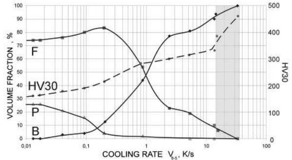
Fig. 5. Influence of the cooling rate on structure and hardness of the cast steel
