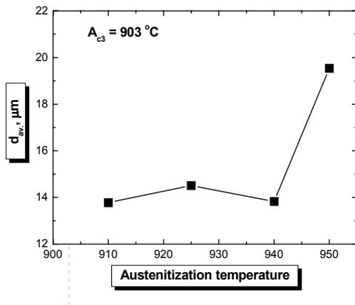
Fig. 3. Changes of the austenite grains mean diameter depending on the austenitization temperature
