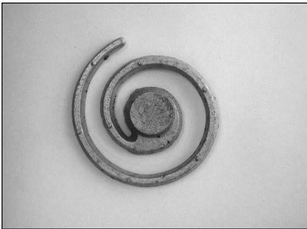
Fig. 4. Spiral cast of AJ62 alloy after pouring from temperature 695°C. Fluidity length is equal 38 cm
