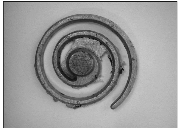
Fig. 5. Spiral cast of AJ62 alloy after pouring from temperature 755°C. Fluidity length is equal 57 cm
