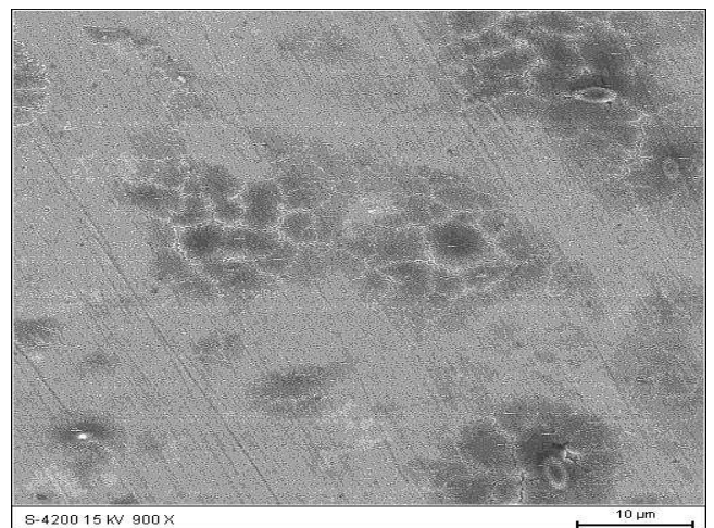
Fig. 3. Evaluation of joint surface condition after corrosion tests in 6% HCl water solution at temperature of 50°C, SEM
