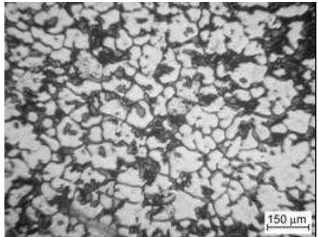
Fig. 1. Microstructure of the as cast ZC63 alloy
