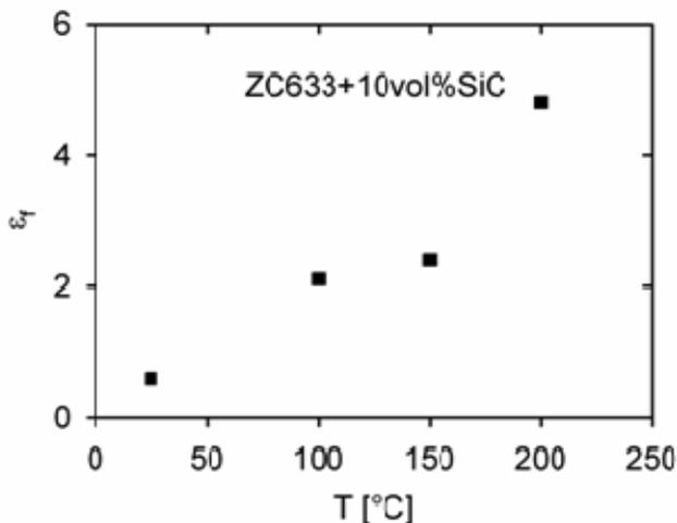
Fig. 4. Temperature dependence of the ductility
