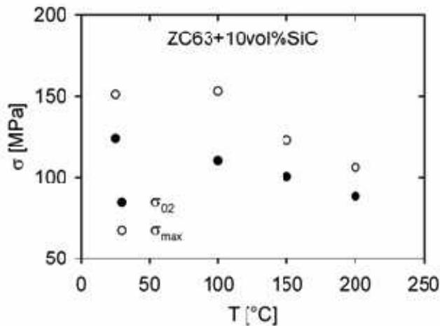
Fig. 3. Temperature dependence of the yield stress and the maximum stress
