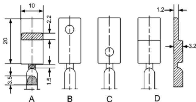
Fig. 1. Injection moulded parts with gates and runners
