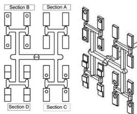
Fig. 2. Layout of parts in the experimental mould
