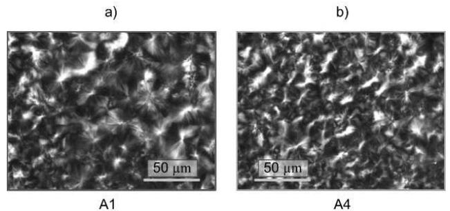
Fig. 6. Spherulitic structure (in core layer) of parts from cavities 1 and 4 in mould section A
