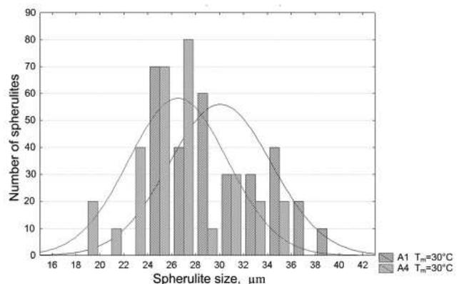
Fig. 7. Spherulite size in the core layer of parts from cavities 1 and 4 in mould section A
