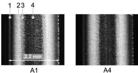
Fig. 5. Morphology of parts from cavities: A1 (left) and A4 (right); 1-skin layer, 2-oriented core zone, 3- transient zone, 4-non-oriented core zone
