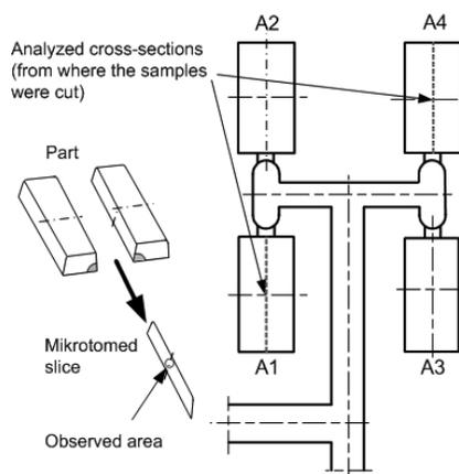
Fig. 3. Samples taken from parts obtained from mould section A
