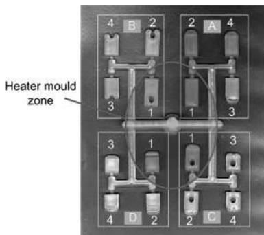
Fig. 4. Short shots made at injection time  $t_i=0,55$  s
