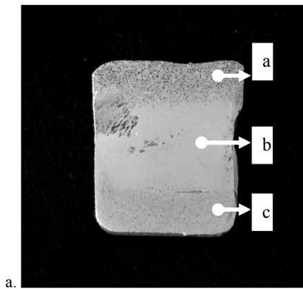
Fig. 2. Macrostructure of AlSi12CuNiMg2/10% SiC 50 $\mu$ m + 10 % Cg. composites with layered particles displacement visible in the matrix.
