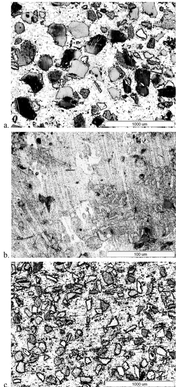
Fig. 4. Microstructure of AlSi12CuNiMg2/10% SiC 50 $\mu$ m + 10 % Cg composite, OM; a) upper part of the composite ingot, b) middle part of the composite ingot, c) lower part of the composite ingot.
