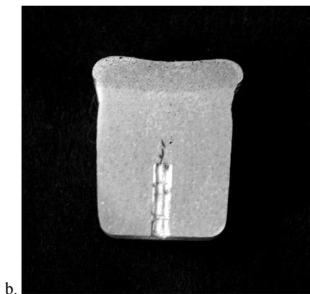
Fig. 3. Macrostructure of AlSi12CuNiMg2 + 20% Cg composites with particles displacement in upper part of the cast visible in the matrix.
