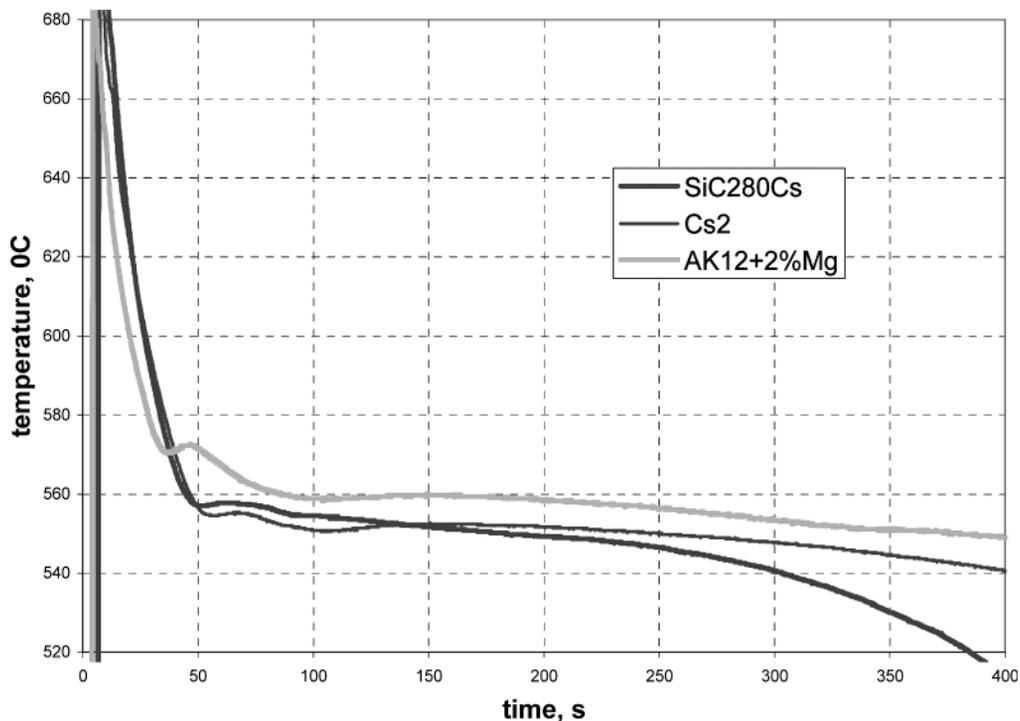
Fig. 1. Solidification curves of aluminium matrix alloy and composites
