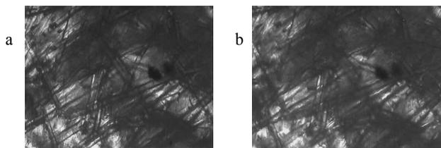
Fig. 6. Structure of PP + 25 % the glass fibre observed on optical microscope during heating in white light with magnification x9 and temperature: a) 30 °C, b) 60 °C
