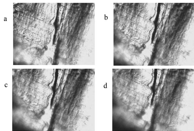
Fig. 4. Structure PP observed on optical microscope during heating in white light with magnification x 9 and temperature: a) 30 °C, b) 60 °C, c) 90 °C, d) 130 °C
