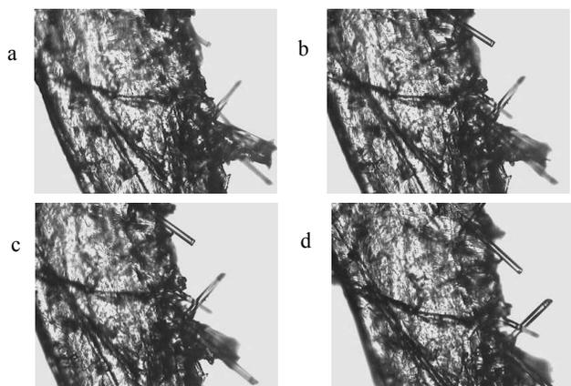
Fig. 5. Structure of PP + 15 % the glass fibre observed on optical microscope during heating in white light with magnification x9 and temperature: a) 30 °C, b) 60 °C, c) 90 °C, d) 130 °C
