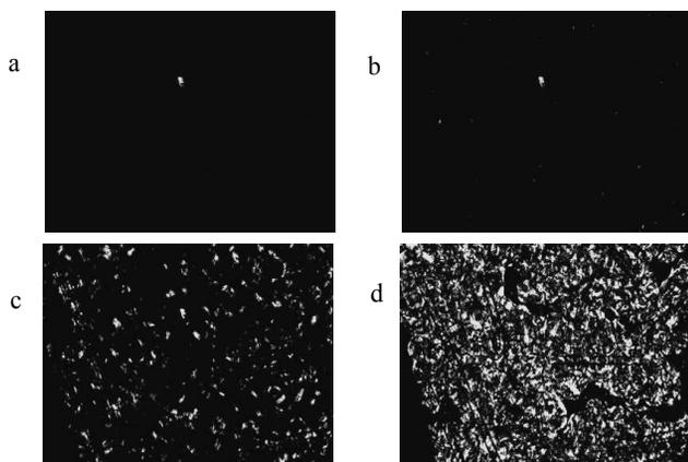
Fig. 2. Structure of PP + 15 % the glass fibre observed on optical microscope during cooling in polarized light and temperature: a) 147 °C, b) 121 °C, c) 117 °C, d) 110 °C
