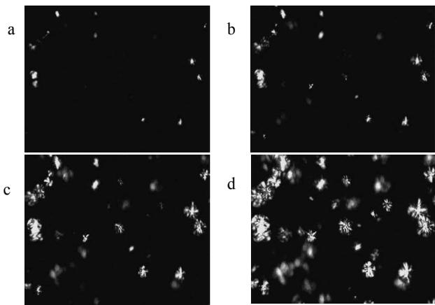
Fig. 1. Structure of PP observed on optical microscope during cooling in polarized light with magnification x 9 and temperature: a) 125 °C, b) 124 °C, c) 123 °C, d) 122 °C
