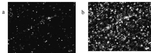
Fig. 3. Structure of PP + 25 % the glass fibre observed on optical microscope during cooling in polarized light with magnification x 9 and temperature: a) 128 °C, b) 126 °C
