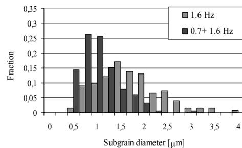
Fig. 9. Subgrain diameter distributions developed in samples 3 and 5
