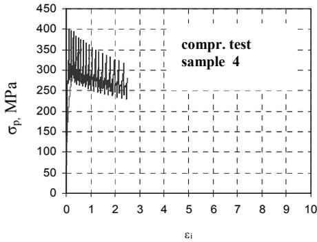
Fig. 3. Stress-strain curves obtained for Al under compression test and combined methods of compression and oscillatory compression at 0.4 Hz
