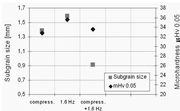
Fig. 10. Subgrain size and microhardness of Al after successive mode of deformation
