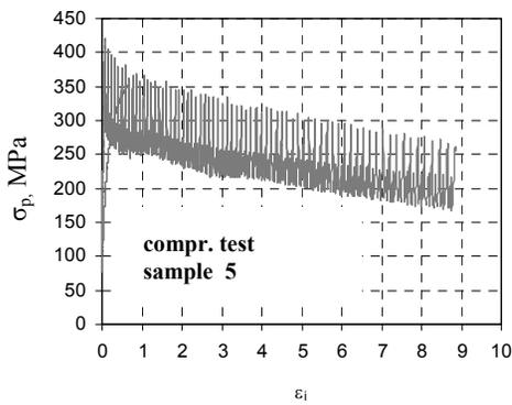
Fig. 4. Stress-strain curves obtained for Al under compression test and combined methods of compression and oscillatory compression at 1.6 Hz
