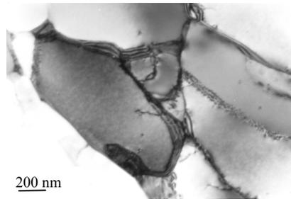
Fig. 7. The microstructure of sample 3. TEM micrograph showing a grain, which is surrounded by a polygonized dislocation wall and by grain boundaries
