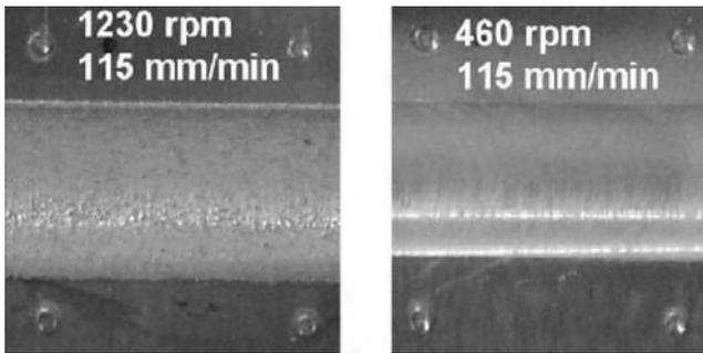
Fig. 6. Surface quality of “hot” and “cold” welds
