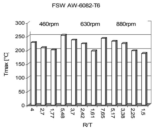
Fig. 3. Maximum temperature as a function of R/T ratio
