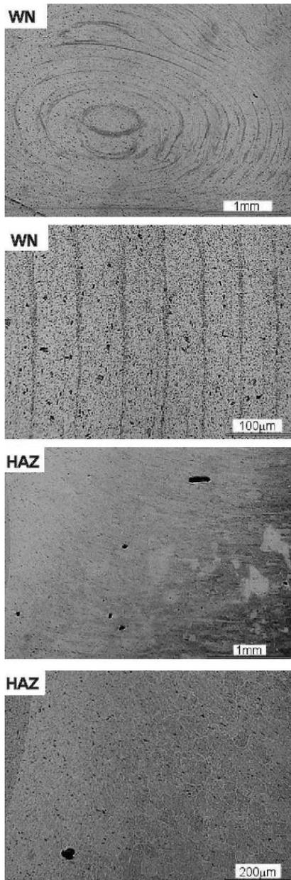
Fig. 12. Microstructures in various zones of the weld FSW-03
