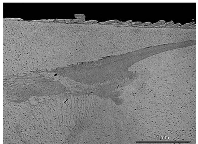
Fig. 14. Flow arm in a FSW weld
