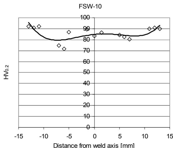
Fig. 11. Hardness profile of the weld FSW-10
