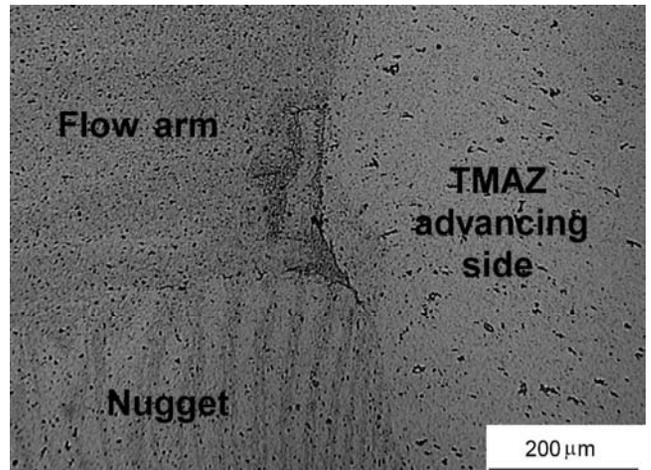
Fig. 13. Initial stage of tunnel defect in the weld FSW-03
