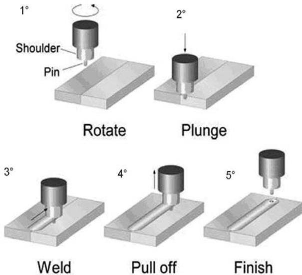
Fig. 1. Schematic representation of FSW process
