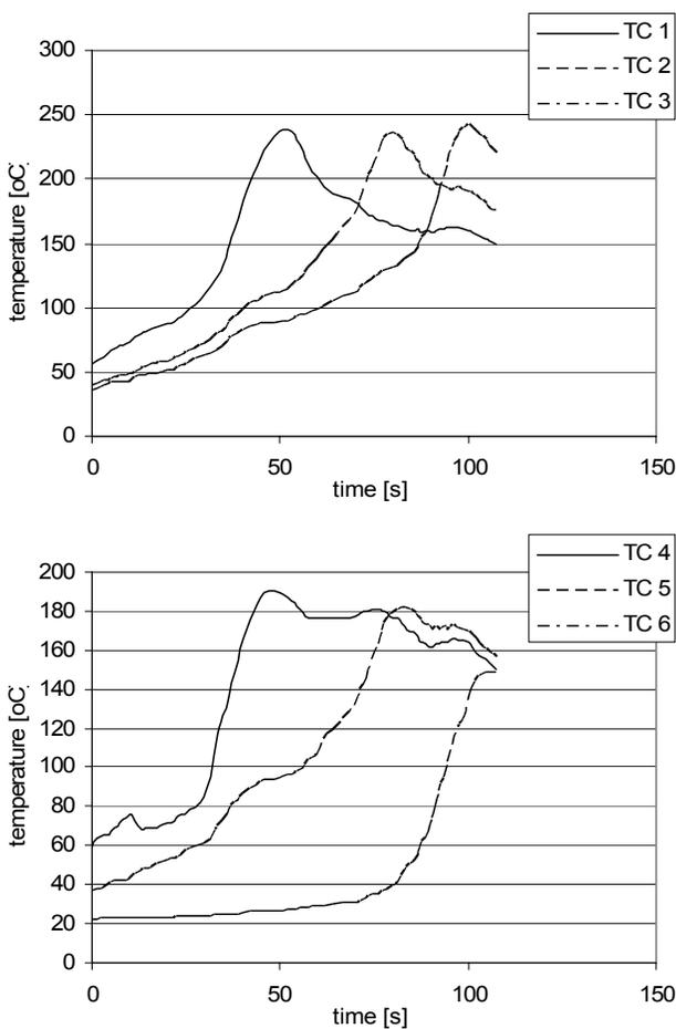
Fig. 2. Temperatures acquired in the weld FSW-02
