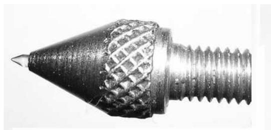
Fig. 2. The measuring cone-shaped end
