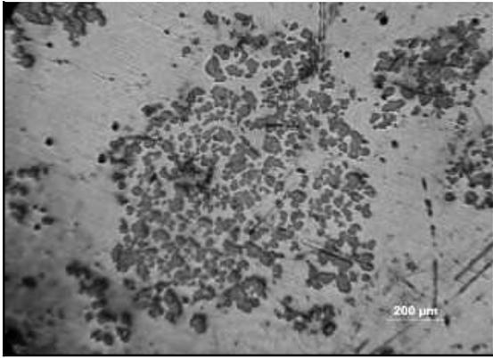
Fig. 5. Silver alloy based composite material reinforced with Fe (200) iron particles structure after the process of chemical silver deposition (the process conducted in the resistance furnace)
