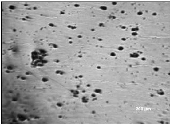
Fig. 6. Silver alloy based composite material reinforced with glass carbon particles Cs (100) after the process of chemical silver deposition
