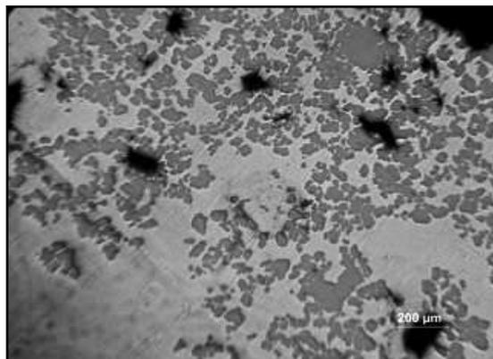
Fig. 4. The structure of silver alloy based composite material reinforced with iron powder Fe (200) after the process of chemical silver deposition (the process conducted in the induction furnace)
