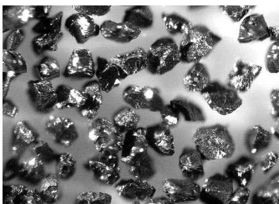
Fig. 3. Glass carbon Cs (100) appearance after the chemical silver deposition processb), optical microscope, mag. 250x
