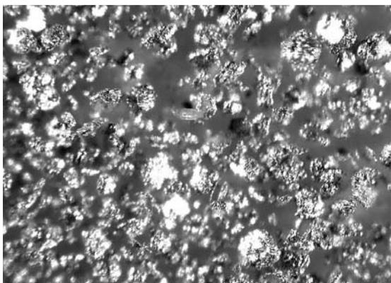
Fig. 2. Iron powder Fe (200) appearance after the chemical silver deposition process; optical microscope, mag. 250x
