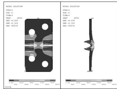
Fig. 6. Stress distribution of rectangular plate with four holes, Von mises criteria is applied (3000N)
