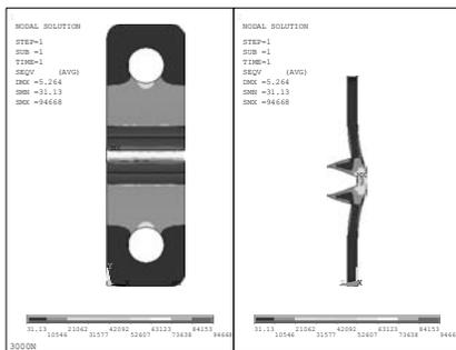
Fig. 5. Stress distribution of rectangular plate with two holes, Von mises criteria is applied (3000N)
