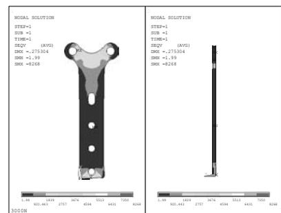
Fig. 7. Stress distribution on the plate with six holes and without wedges, Von mises criteria is applied (3000N)
