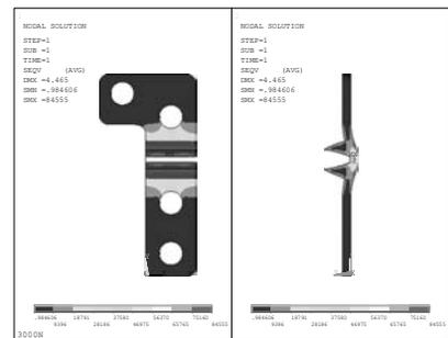
Fig. 8. Stress distribution of the L shaped plate with four holes, Von mises criteria is applied (3000N)
