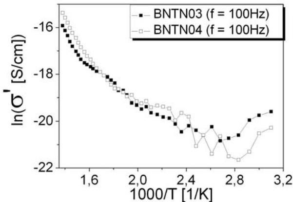
Fig. 6. The ac-conductivity dependence on reciprocal temperature for 100Hz frequency of measuring field taken under cooling for BNTN03 and BNTN04 samples
