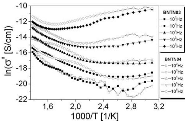
Fig. 5. The ac-conductivity dependence on reciprocal temperature, taken under cooling for BNTN03 and BNTN04 samples
