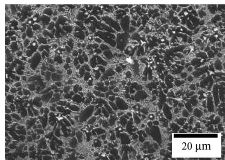
Fig. 6. Microstructure of the 32CrMoV12-28 steel remelted with TiC powder with laser power 2.0kW
