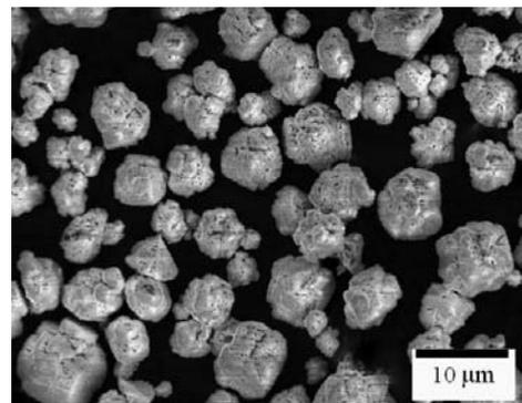
Fig. 3. Aluminium oxide  $\text{Al}_2\text{O}_3$  ceramic powder using for alloying with the hot work tool steel
