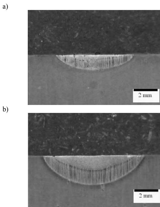
Fig. 4. Shape and thickness of cross-section of the laser remelted samples Al<sub>2</sub>O<sub>3</sub> a) 1.2 kW, b) 2.3 kW
