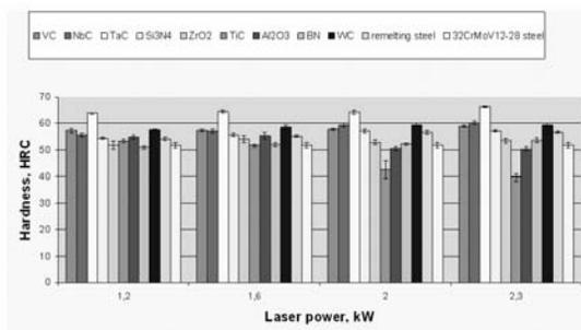
Fig. 7. Hardness measurements results (HRC) of the remelted and alloyed surface
