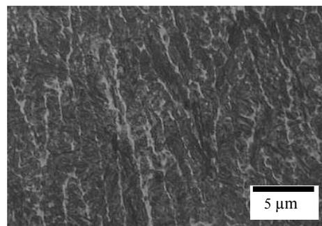
Fig. 5. Microstructure of the 32CrMoV12-28 steel remelted with ZrO<sub>2</sub> powder with laser power 2.0kW
