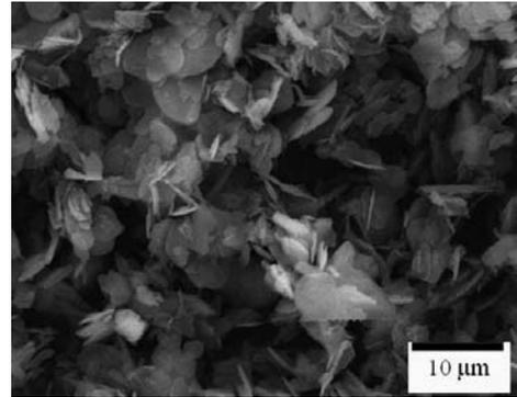
Fig. 1. Boron nitride BN ceramic powder using for alloying with the hot work tool steel
