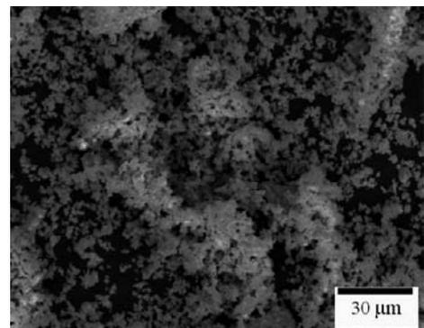
Fig. 2. Tantalum carbide TaC ceramic powder using for alloying with the hot work tool steel
