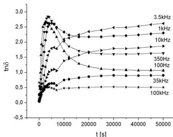
Fig. 6. The effective energy loss factor of maize-starch granules population as a function of time for 7 selected frequencies. It was measured as the response on the step of ambient atmosphere (0  $\div$   $\sim 100\%$ ) relative humidity at about  $t \approx 0$ s
