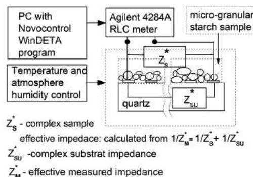
Fig. 3. The effective complex impedance measurement principle and scheme for micro – granular matter (starch) placed on the interdigitated electrode sensor
