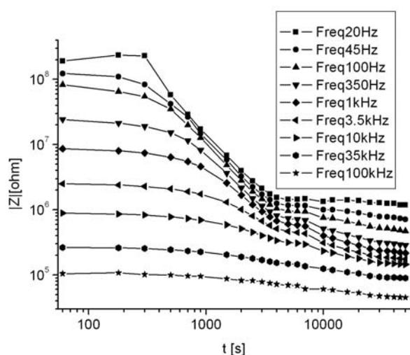
Fig. 7. The absolute value of electric effective impedance ( $|Z^*|$ ) evolution measured as response on the step of ambient atmosphere relative humidity step ( $0 \div \sim 100\%$ ) at room temperature
