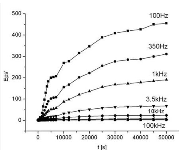
Fig. 5. The effective dielectric permittivity ( $\text{Eps}'$ ) of maize-starch granules sample as a function of time for 9 selected frequencies. It was measured as the response on the step of ambient atmosphere relative humidity (RH) from 0 to  $\sim 100\%$  at room temperature. The RH step was initiated for  $t=0$ s
