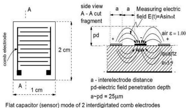
Fig. 1. The interdigitated – comb dielectric sensor geometry: front and side view cut of substrate and metallic electrodes
