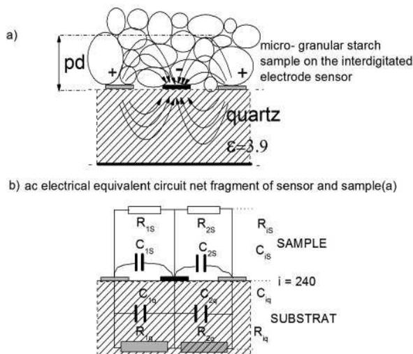
Fig. 2. a) micro – granular matter (starch) sample on the interdigitated electrode sensor, b) ac – electrical equivalent circuit – net fragment of sensor (substrate) and micro – granular sample placed on the sensor surface
