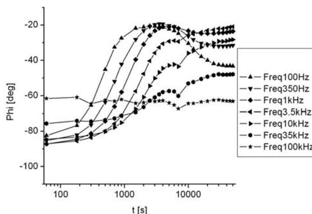
Fig. 8. Time and frequency dependence of effective phase angle ( $\Phi$ [deg]) for maize starch granules population measured as response on ambient atmosphere relative humidity step  $0 \div \sim 100\%$  at room temperature
