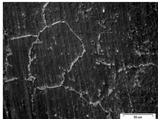
Fig. 2. Microstructure of supersaturated Mg-7Al-3Nd alloy (LM)
