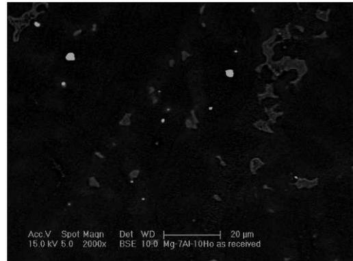
Fig. 9. Microstructure of as-cast Mg-7Al-10Ho alloy (BSE)
