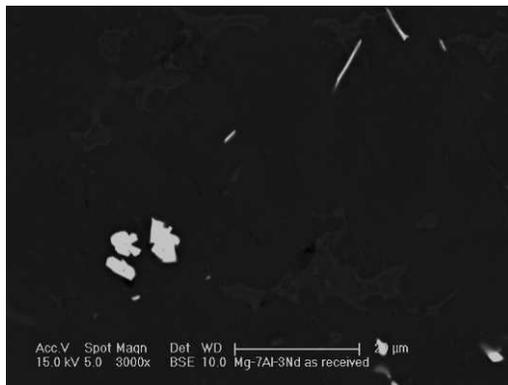
Fig. 4. Microstructure of as-cast Mg-7Al-3Nd alloy (BSE)
