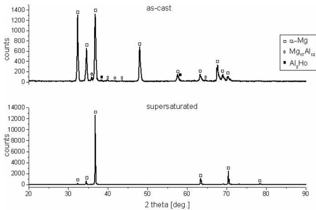
Fig. 8. X-ray diffraction pattern of as-cast and supersaturated Mg-7Al-10Ho alloy
