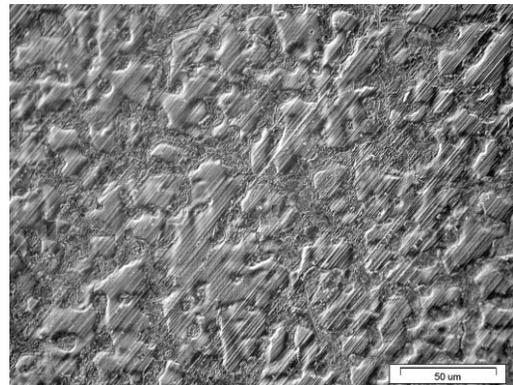
Fig. 1. Microstructure of as-cast Mg-7Al-3Nd alloy (LM)
