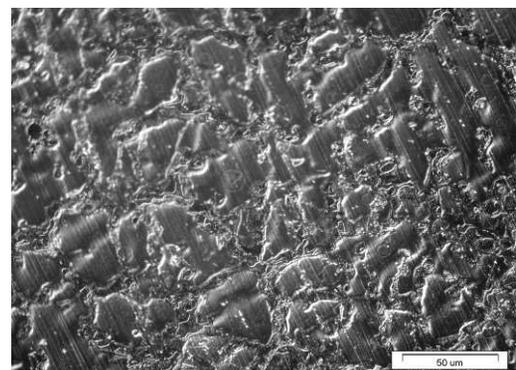
Fig. 6. Microstructure of as-cast Mg-7Al-10Ho alloy (LM)
