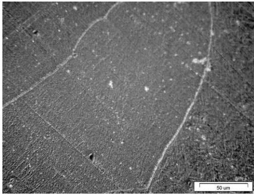
Fig. 7. Microstructure of supersaturated Mg-7Al-10Ho alloy (LM)
