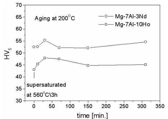
Fig. 11. The Vickers hardness changes during aging at 200°C for Mg-7Al alloys with 3% Nd and 10% Ho addition
