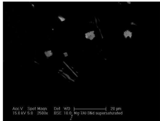
Fig. 5. Microstructure of supersaturated Mg-7Al-3Nd alloy (BSE)
