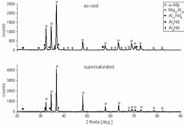
Fig. 3. X-ray diffraction pattern of as-cast and supersaturated Mg-7Al-3Nd alloy
