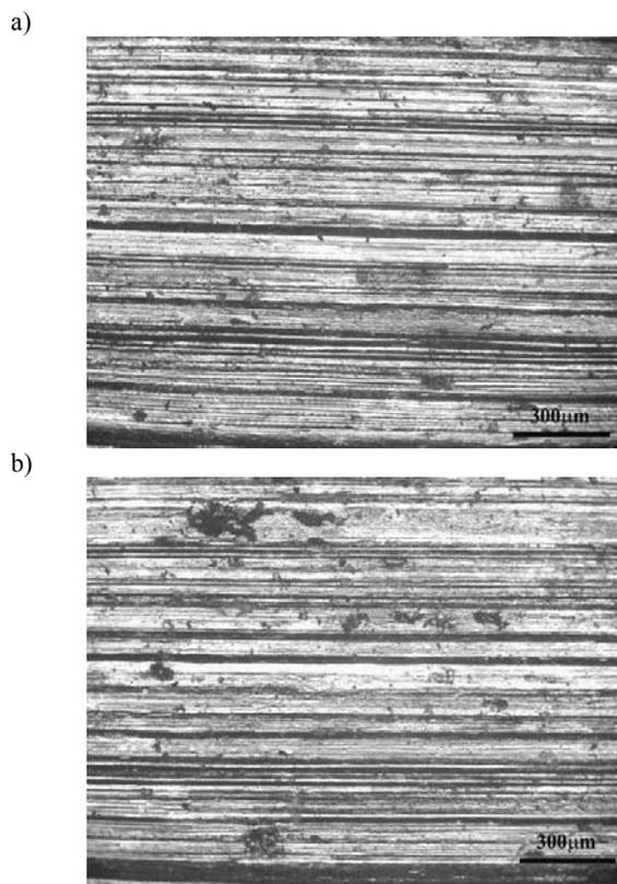
Fig. 10. Overall wear surface of composites containing 1.9 % of graphite fibres and 6.5 % of Al<sub>2</sub>O<sub>3</sub> at 0.81 MPa load (a), and 1.35 MPa load (b).
