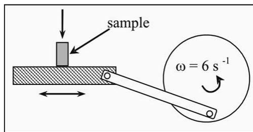
Fig. 2. Diagram of the tribological test stand
