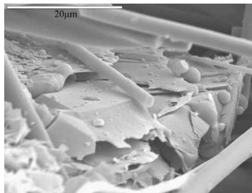
Fig. 1. Fracture of a preform with graphite flake and binder drops on it
