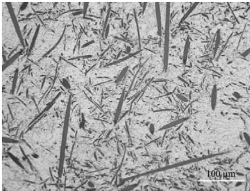
Fig. 5. Microstructure of hybrid composite material reinforced with  $\text{Al}_2\text{O}_3$  and graphite fibers
