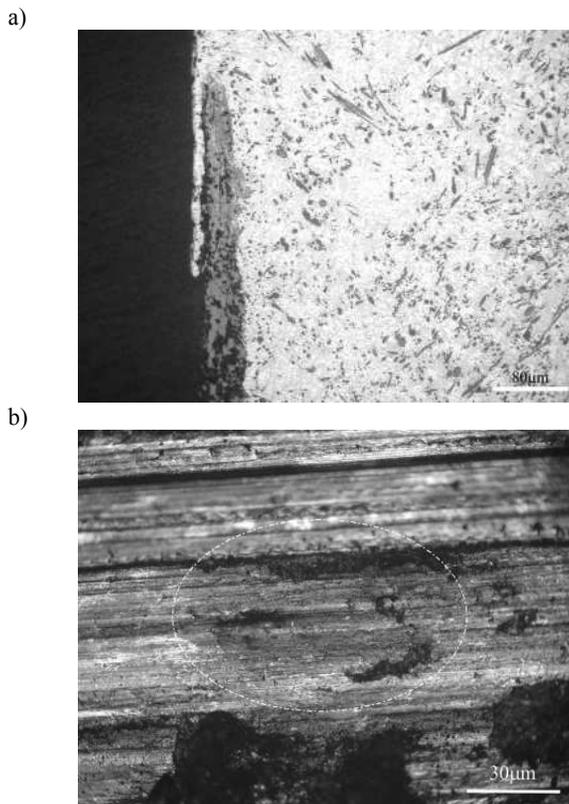
Fig. 14. Covering of cavity with debris (a), crack of scale over closed cavity (b)
