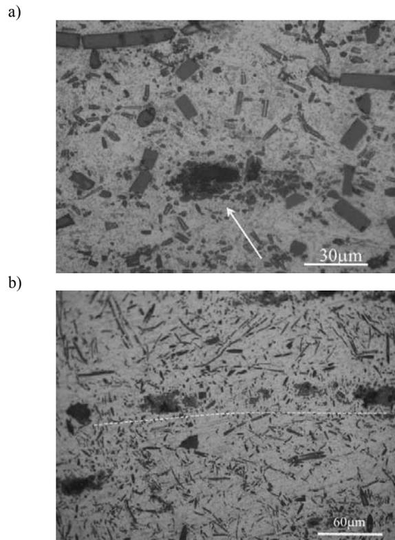
Fig. 12. View of a crumbled graphite fibre (a), connection of the erode places along the wear direction (b)
