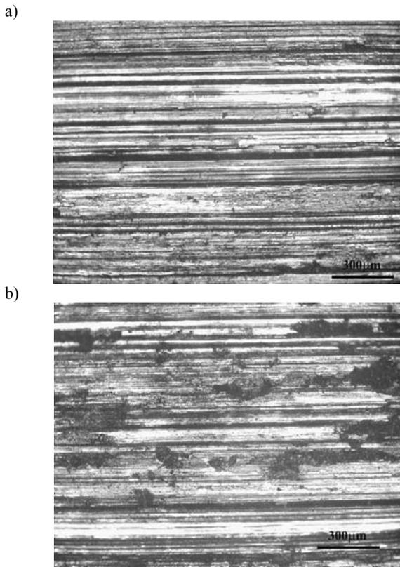
Fig. 11. Overall wear surface of composites containing 13.6 % of graphite flakes and 7.4 % of  $\text{Al}_2\text{O}_3$  at 0.81 MPa load (a), and 1.35 MPa load (b)
