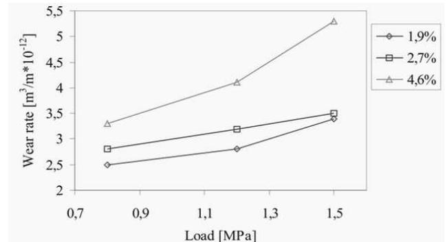
Fig. 7. Effect of pressure on wear of composite with constant 8 % of  $\text{Al}_2\text{O}_3$  and 1.9 - 2.7 - 4.6 % of graphite fibres
