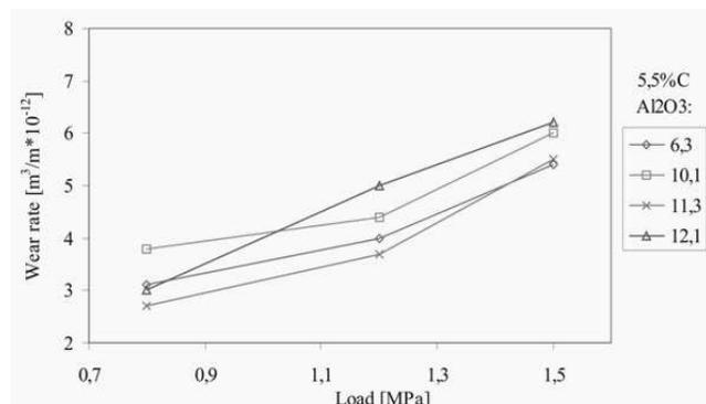
Fig. 9. Effect of pressure on wear of composite with constant 5.5 % of graphite flakes and 6.3 – 10.1 – 11.3 – 12.1 % of Al<sub>2</sub>O<sub>3</sub> fibres
