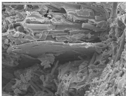
Fig. 3. Fracture of the composite with a graphite flake
