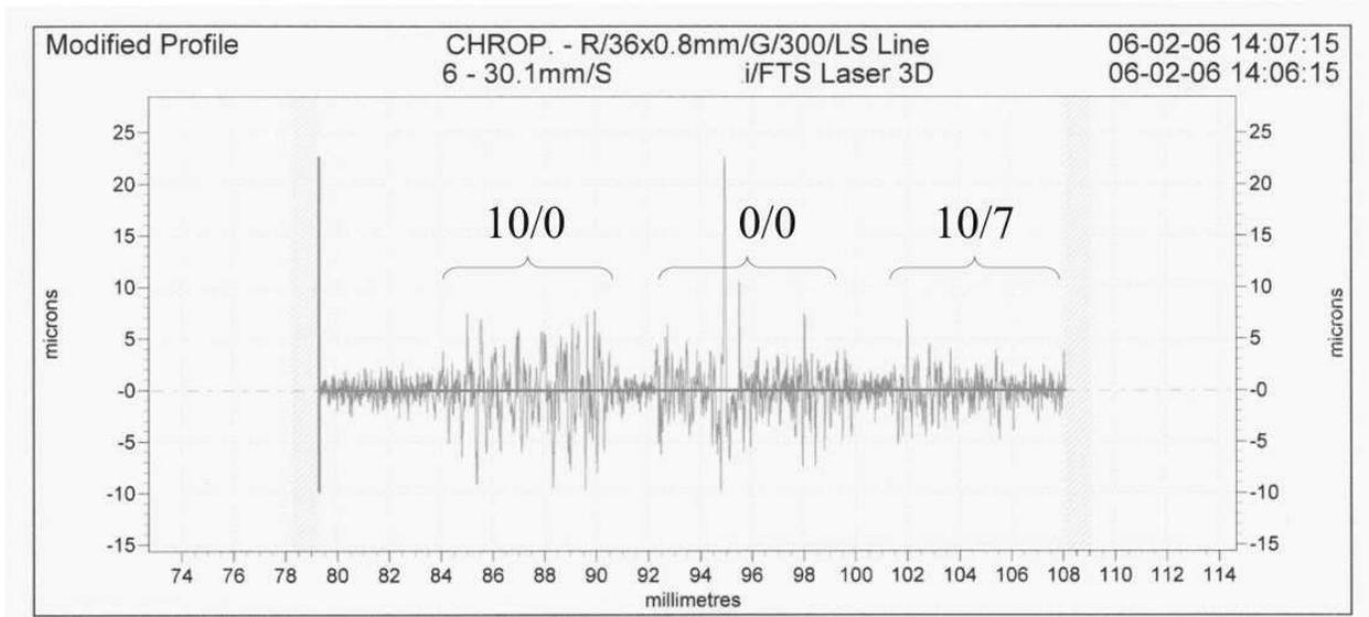
Fig. 15. Profile of counterpart after test with composite, unreinforced alloy and hybrid composite
