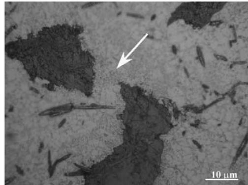
Fig. 4. Microstructure of hybrid composites with the view of partly uncovered single graphite flake
