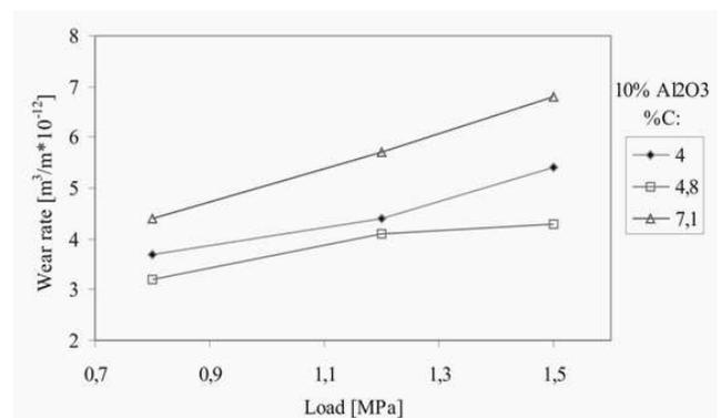
Fig. 8. Effect of pressure on wear of composite with constant 10 % of  $\text{Al}_2\text{O}_3$  and 4.0 - 4.8 - 7.1 % of graphite flakes
