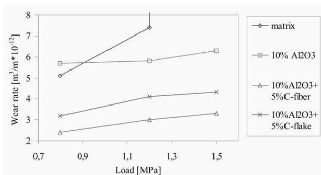
Fig. 6. Effect of pressure on wear of unreinforced alloy, composite with 10 % of  $\text{Al}_2\text{O}_3$  fibres, composite with 10 % of  $\text{Al}_2\text{O}_3$  fibres and 5 % of graphite fibres, composite with 10 % of  $\text{Al}_2\text{O}_3$  fibres and 5 % of graphite flakes at  $P_2 = 1.35$  MPa
