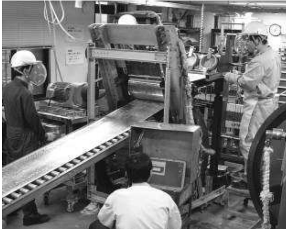
Fig. 4. Twin roll casting in operation at 20m/min
