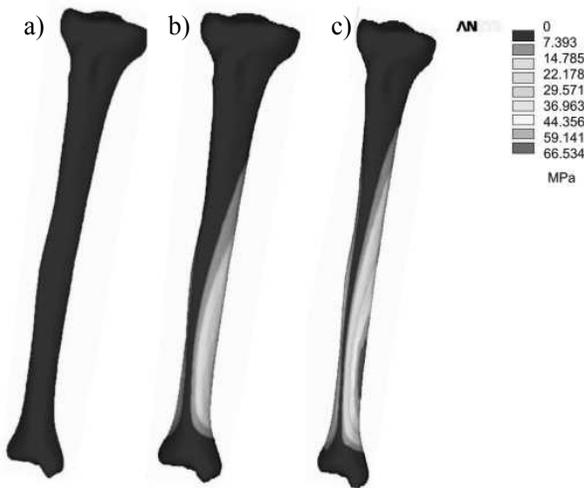
Fig. 4. Stresses in the healthy tibia loaded with the force: a) 100N, b) 1000N, c) 2000N
