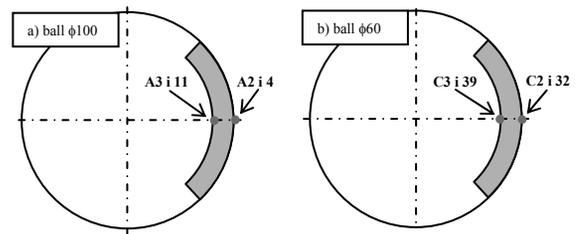
Fig. 1. The position of measurement points: A3, A2, C3, C2 –thermoelements in experiment; 1, 4, 39, 32 – thermoelements in simulation
