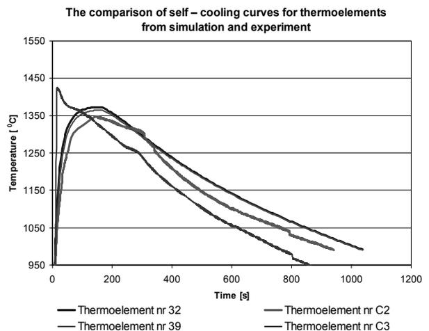
Fig. 3. Self - cooling curves for ball  $\phi 60$  in measurement points of the premould surface placed on the outer side (nr 32 and C 2), on the inner side (nr 39 and C 3),  $T_{zal} = 1550^{\circ}C$
