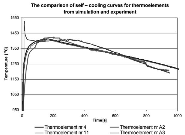
Fig. 2. Self - cooling curves for ball  $\phi 100$  in measurement points of the premould surface placed on the outer side (nr 4 and A 2), on the inner side (nr 11 and A 3),  $T_{zal} = 1550^{\circ}C$
