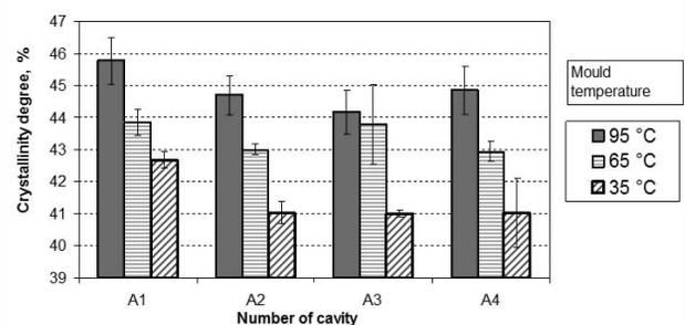
Fig. 4. Crystallinity degree for samples from different cavities
