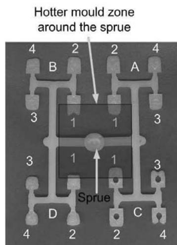
Fig. 1. Short shots into the multicavity mould – inequality of cavities' filling; A-D: cavity sections; 1-4: filling sequence
