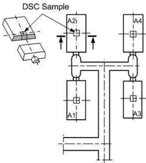
Fig. 2. Cutting out of samples from injection moulded parts
