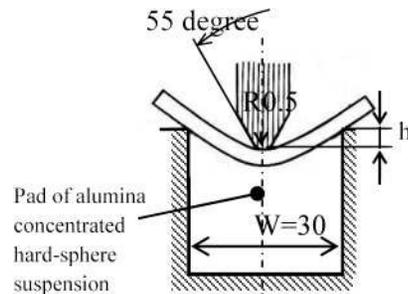
Fig. 6. V-bending with alumina concentrated hard-sphere suspension pad
