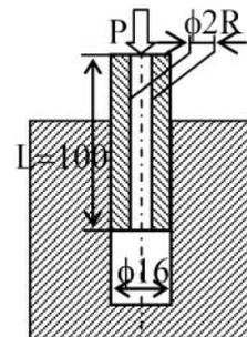
Fig. 3. Backward extrusion test
