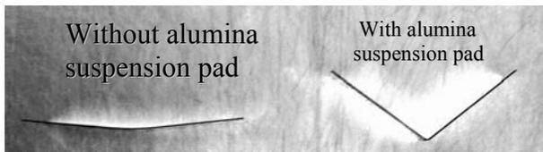
Fig. 7. V-bending samples. The left one is a sample of partial bending without the alumina suspension pad (air bending), and the right one is with it
