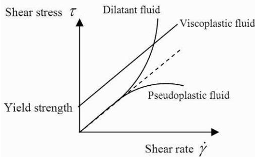
Fig. 1. Typical non-Newtonian fluid
