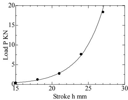
Fig. 8. Punch stroke and forming load
