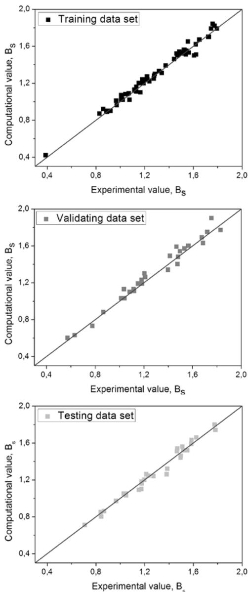
Fig. 3. Comparison of the experimental and calculated  $B_s$  values for MLP 15-5-1 network sets: training, validating, testing
