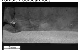
EnDOTec DO*33 microstructure: iron alloy based complex metal borides and carbides
