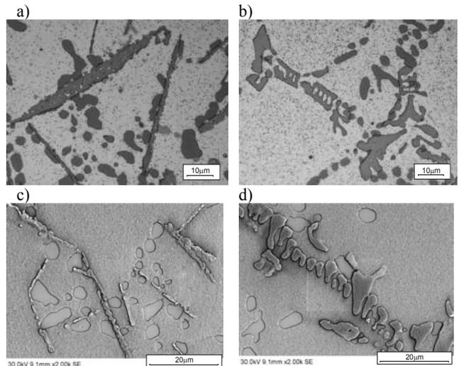
Fig. 1. The microstructure of the AlSi5Cu2Mg alloy in the T6 condition a and b) images form light microscope (LM), c and d) images from scanning electron microscope (SEM)
