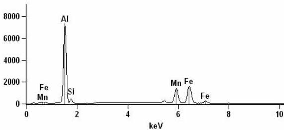
Fig. 3. The EDS spectrum of the “Chinese script” shaped inclusions local analysis
