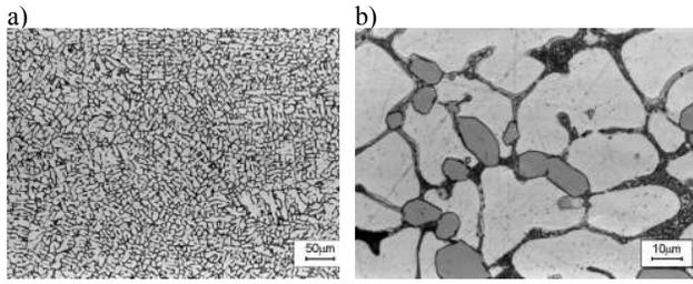
Fig. 8. The AlSi5Cu2Mg alloy microstructure after 20 minutes annealing at 629°C
