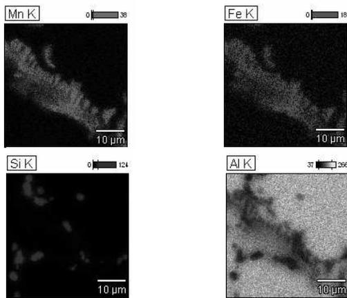
Fig. 2. The surface distribution of the alloying elements in the area of Si and “Chinese script” shaped inclusions occurrence
