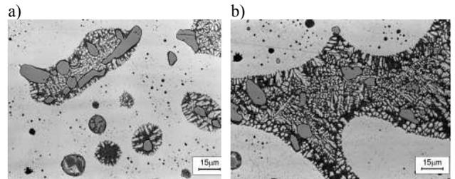
Fig. 6. The AlSi5Cu2Mg alloy microstructure after 20 minutes annealing at 568°C
