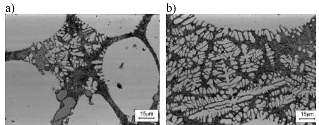
Fig. 7. The AlSi5Cu2Mg alloy microstructure after 20 minutes annealing at 580°C
