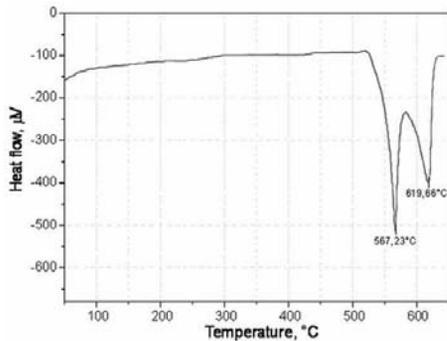
Fig. 4. DSC thermogram of the AlSi5Cu2Mg alloy in the T6 conditions to the temperature 625°C at the rate of 4°C/min
