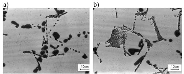
Fig. 5. The AlSi5Cu2Mg alloy microstructure after 20 minutes annealing at 518°C
