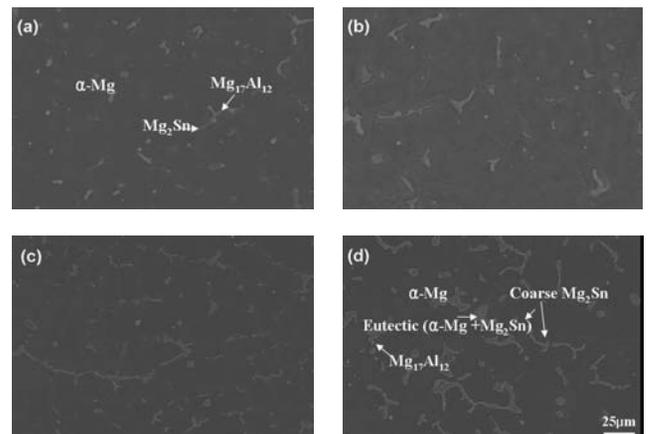
Fig. 2. SEM microscopy microstructures of the Mg-xSn-5Al-1Zn alloy (a) 5wt% Sn (b) 8wt% Sn
