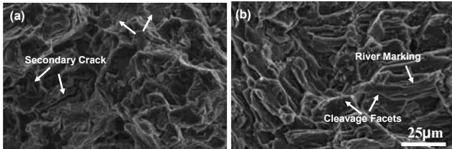
Fig. 8. Factography of Mg-xSn-5Al-1Zn alloys by tensile fracture: (a) 5wt%Sn (b) 8wt%Sn
