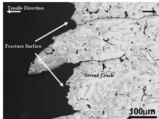
Fig. 6. Optical result for the vertical section of the TAZ551 specimen failed in tensile test
