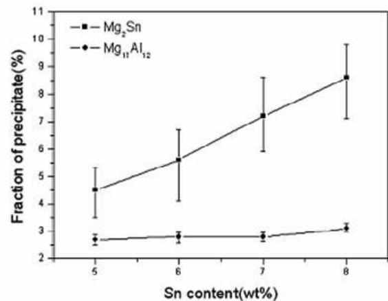
Fig. 3. Mg-xSn-5Al-1Zn alloys volume percentage of precipitates of Mg<sub>2</sub>Sn and Mg<sub>17</sub>Al<sub>12</sub>
