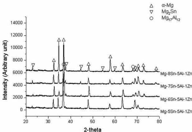
Fig. 1. XRD patterns of Mg-xSn-5Al-1Zn alloys
