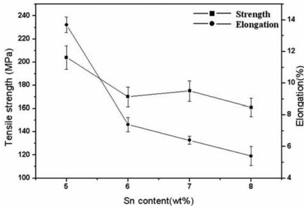
Fig. 4. Tensile properties of Mg-xSn-5Al-1Zn alloys in as-cast at room temperature
