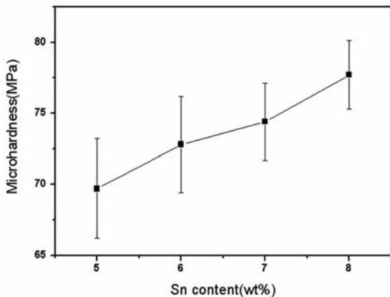
Fig. 5. Micro hardness of Mg-xSn-5Al-1Zn alloys in as-cast (x: 5, 6, 7, 8 wt%)
