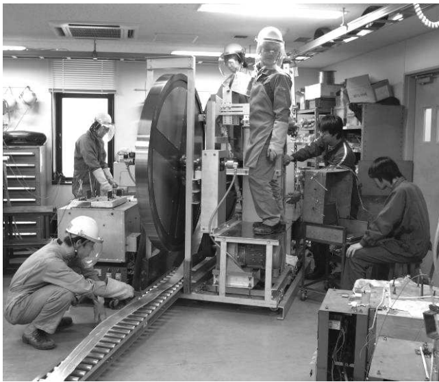
Fig. 2. Roll caster in operation. A high speed twin roll caster equipped with 1500 mm diameter rolls
