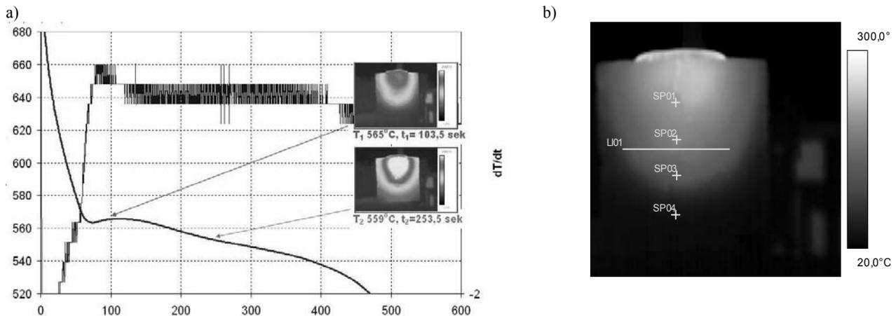
Fig. 2. The AK12/ SiC+C composite: a) solidification curve of composite solidify in a sand mould, b) thermal image and temperature profile on the outside surface of sand mould; start of solidification: T1 565oC, t1= 103,5 s
