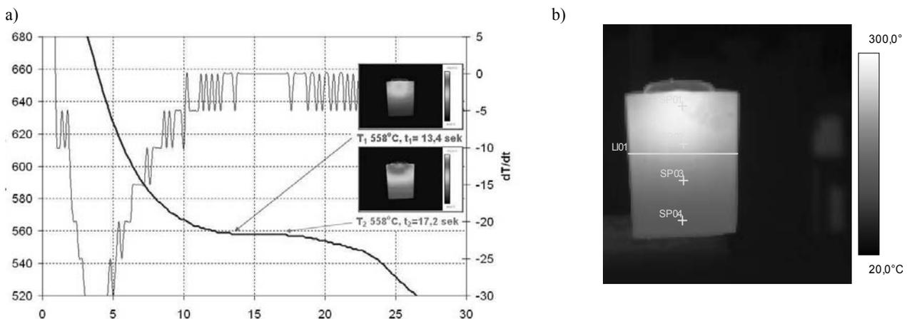
Fig. 1. The AK12/ SiC+C composite: a) solidification curve of composite solidify in a graphite mould, b) thermal image and temperature profile on the outside surface of graphite mould; start of solidification:  $T_1 = 558^\circ\text{C}$ ,  $t_1 = 13,4$  s
