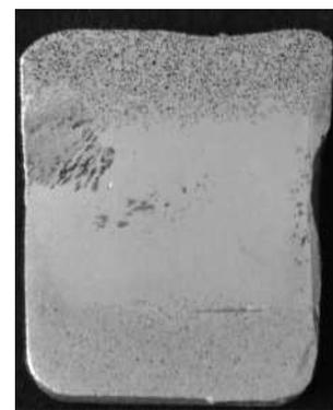
Fig. 4. The macrostructure of AK12/ SiC+C composite solidified in a sand mould; the layered displacement of ceramic particles in the matrix is visible on the picture, [18]
