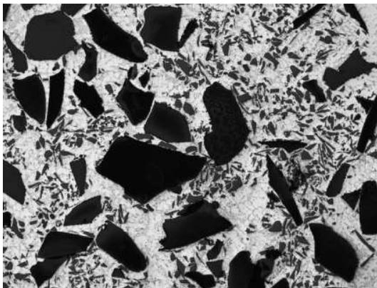
Fig. 3. The microstructure of AK12/ SiC+C composite solidified in a graphite mould, mag. 250x, OM
