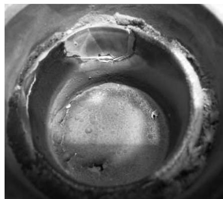
Fig. 1. Reaction chamber interior after 1 hour nitriding process
