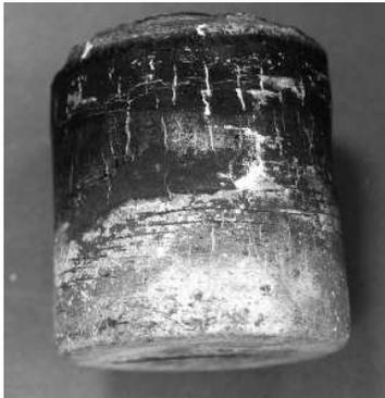
Fig. 3. Ingot after 1 MPa nitriding process
