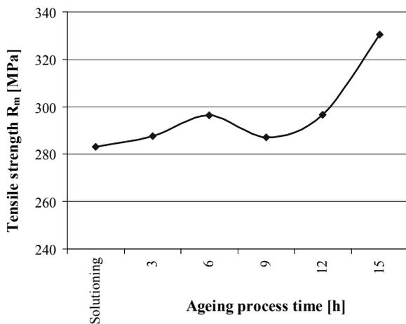
Fig. 6. Tensile strength changed depending on the heat treatment parameters
