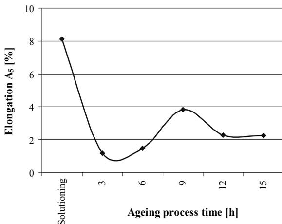
Fig. 7. Elongation changed depending on the heat treatment parameters
