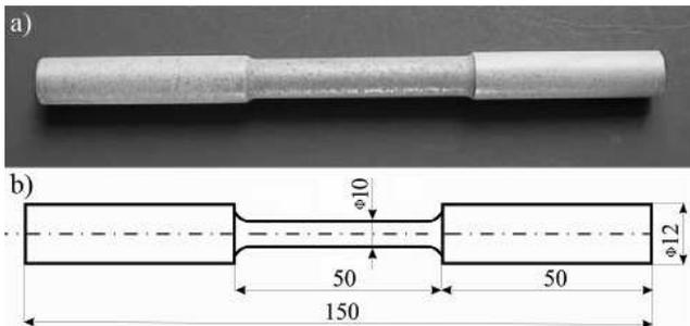
Fig. 1. a) photo of the test specimen, b) line drawing of the sample
