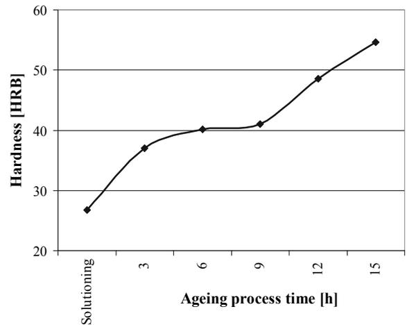
Fig. 4. Hardness changed depending on the heat treatment parameters
