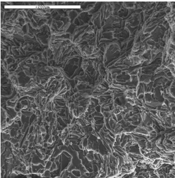
Fig. 3. Fracture of AlSi9Mg alloy after ageing in 150°C by 15 hours
