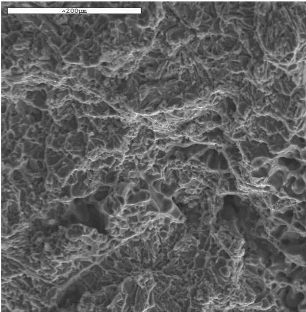
Fig. 2. Fracture of AlSi9Mg alloy after solutioning process where temperature was 530°C and time 6 hours
