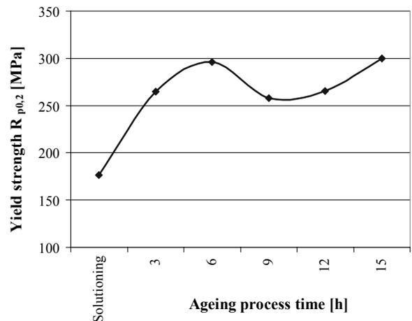
Fig. 5. Field strength changes depending on the heat treatment parameters
