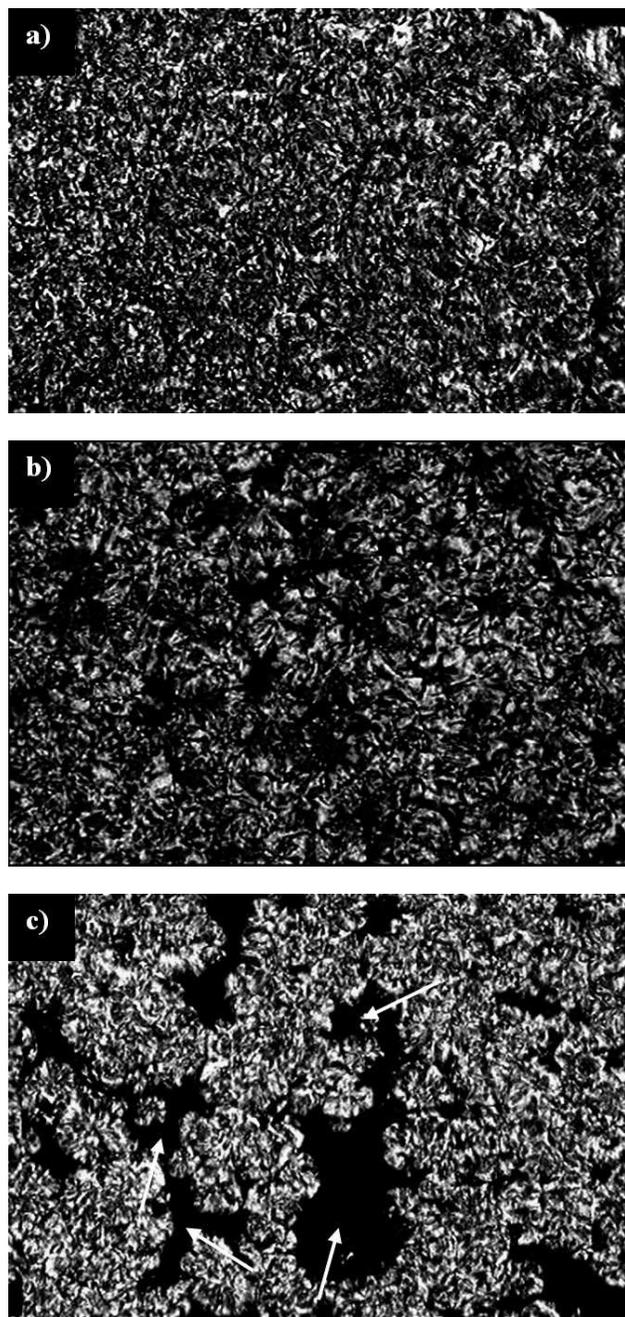
Fig. 2. Morphology of polyoxymethylene (POM) samples in different cooling rates: a) 5°C/min, b) 10°C/min, c) 20°C/min
