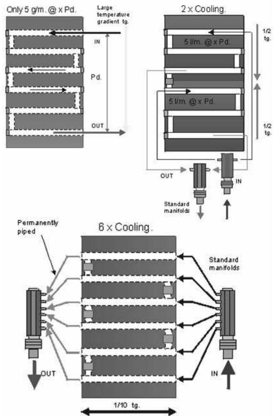
Fig. 1. Three different approaches to cooling channels in the same mould: a) typical joining of cooling channels, b) two-way manifolds, c) two mould mounted manifolds [6]
