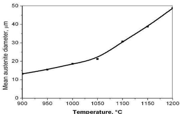
Fig. 2. Influence of austenitizing temperature on a grain size of primary austenite
