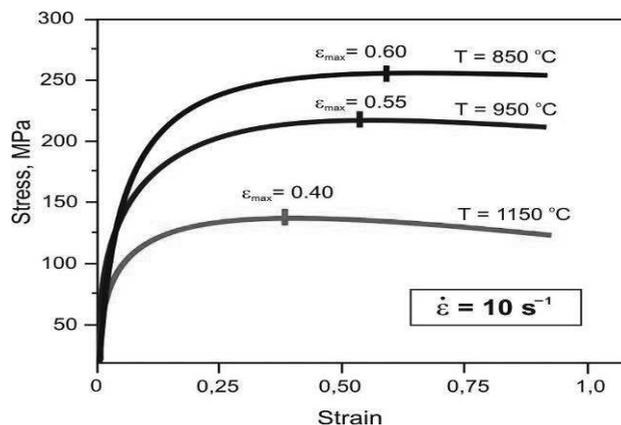
Fig. 7. Influence of temperature on stress-strain curves of the specimens compressed at a strain rate of 10s<sup>-1</sup>
