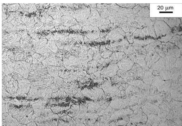
Fig. 3. Structure of primary austenite of the specimen water-quenched from a temperature of 1000°C
