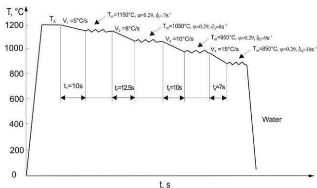
Fig. 1. Conditions of multi-stage hot-compression test
