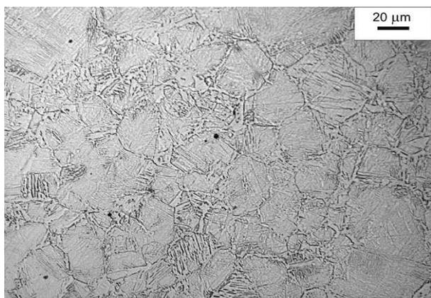
Fig. 4. Structure of primary austenite of the specimen water-quenched from a temperature of 1100°C
