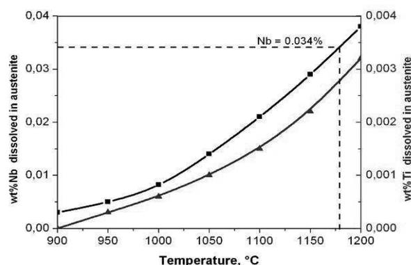
Fig. 5. Temperature dissolution (precipitation) kinetics for TiN ( $\blacktriangle$ ) and NbC ( $\blacksquare$ ) in austenite
