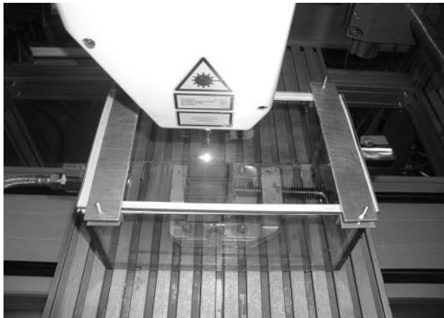
Fig. 4. A view of laser alloying (gas nitriding) of titanium alloy Ti6Al4V in a gas chamber filled in with argon and nitrogen mixture
