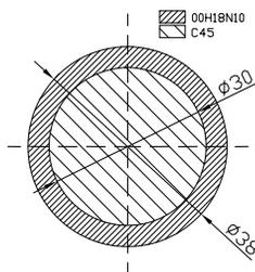
Fig. 5. Form and dimension of bimetallic band
