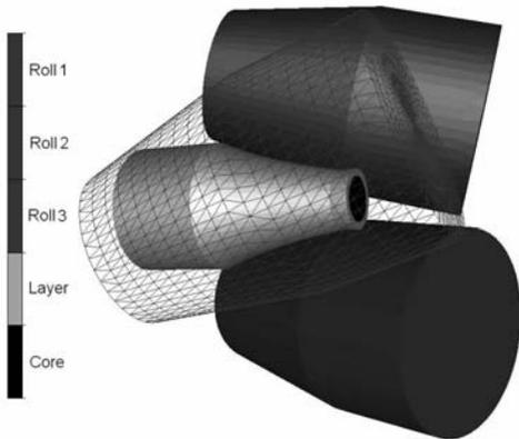
Fig. 4. The rolls and bimetallic band with a finite-element mesh adopted for the simulation of the process of rolling in the three-high skew mill
