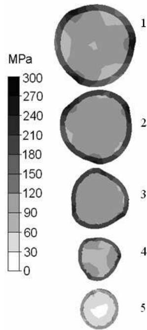
Fig. 6. Distribution of stress intensities: 1) in the plane of entry to the roll gap; 2) in the 1/3 central zone of the roll gap; 3) in the 1/2 central zone of the roll gap; 4) in the 2/3 central zone of the roll gap; 5) in the plane of exit from the roll gap
