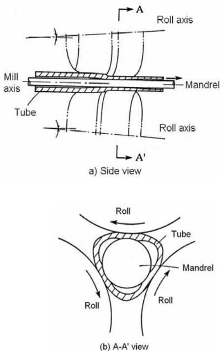
Fig. 1. Schematic view of rotary rolling in elongating process of manufacturing a seamless tube [2]
