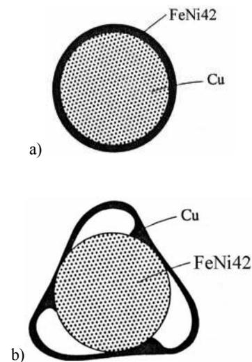
Fig. 2. Effect of deformation resistance on rotary rolling for clad bar[2]; a) Outside layer: FeNi42, Core: Cu; b) Outside layer: Cu, Core: FeNi42
