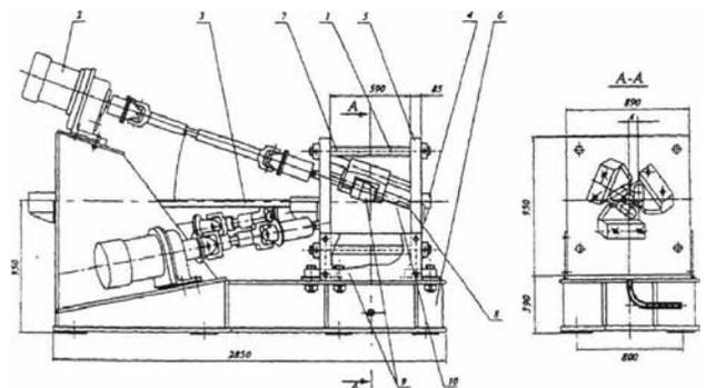
Fig. 3. Three - high skew rolling mill [5], 1 - Working stand, 2 - Primary engine, 3 - Entry guide, 4 - Stripper guide, 5 - Steel plate, 6 - Base, 7 - Distance screws, 8 - Cassettes, 9 - Working rolls, 10 - Thrust bearing
