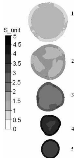
Fig. 7. Distribution of strain intensities: 1) in the plane of entry to the roll gap; 2) in the 1/3 central zone of the roll gap; 3) in the 1/2 central zone of the roll gap; 4) in the 2/3 central zone of the roll gap; 5) in the plane of exit from the roll gap
