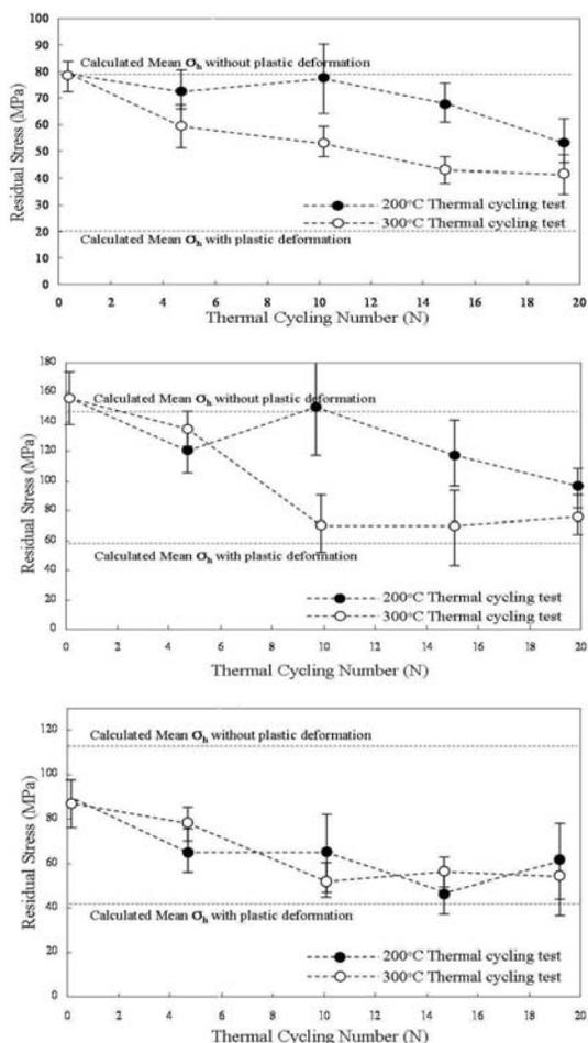
Fig. 6. Residual stress as function of numbers of cycles in AS52/Al<sub>18</sub>B<sub>4</sub>O<sub>33</sub> MMCs, measured by XRD, (a) 15 vol.%, (b) 25 vol.% and (c) 35 vol.%
