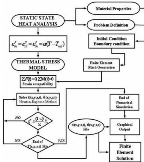
Fig. 3. Flow chart for the numerical modelling of the thermal stresses during thermal cycling test
