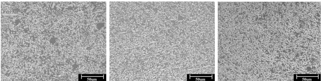
Fig. 4. SEM microscope of AS52/ Al<sub>18</sub>B<sub>4</sub>O<sub>33</sub> MMCs, (a) 15 vol.%, x500, (b) 25 vol.%, x500 and (c) 35 vol.%, x500
