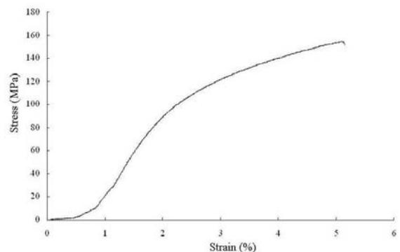
Fig. 2. Stress-Strain curve of AS52 monolithic alloy, at 25°C
