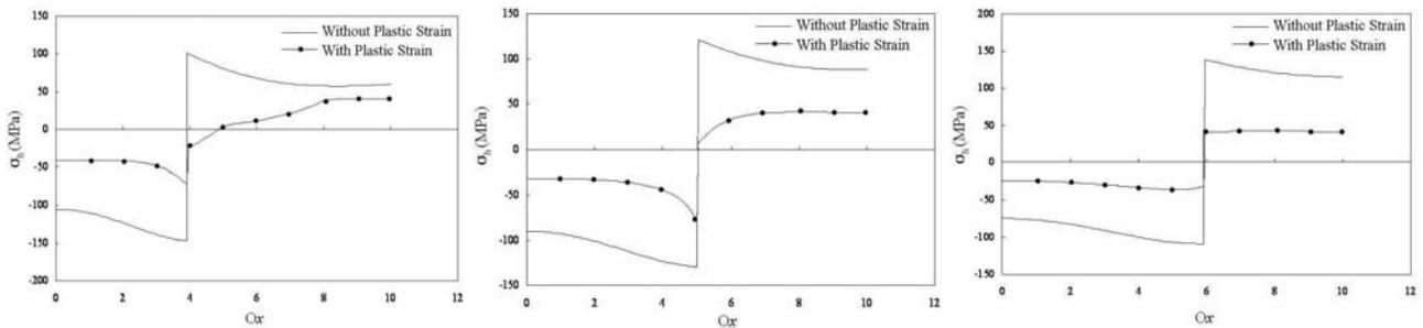
Fig. 5. Profiles of hydrostatic stress component  $\sigma_h$  registered along Ox, for the simulations performed with and without plastic strain in matrix phases, (a) 15 vol.%, (b) 25 vol.% and (c) 35 vol.%
