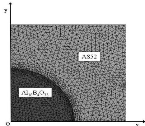
Fig. 1. Representative meshed unit cell of 35% AS52/ $\text{Al}_{18}\text{B}_4\text{O}_{33}$  MMCs
