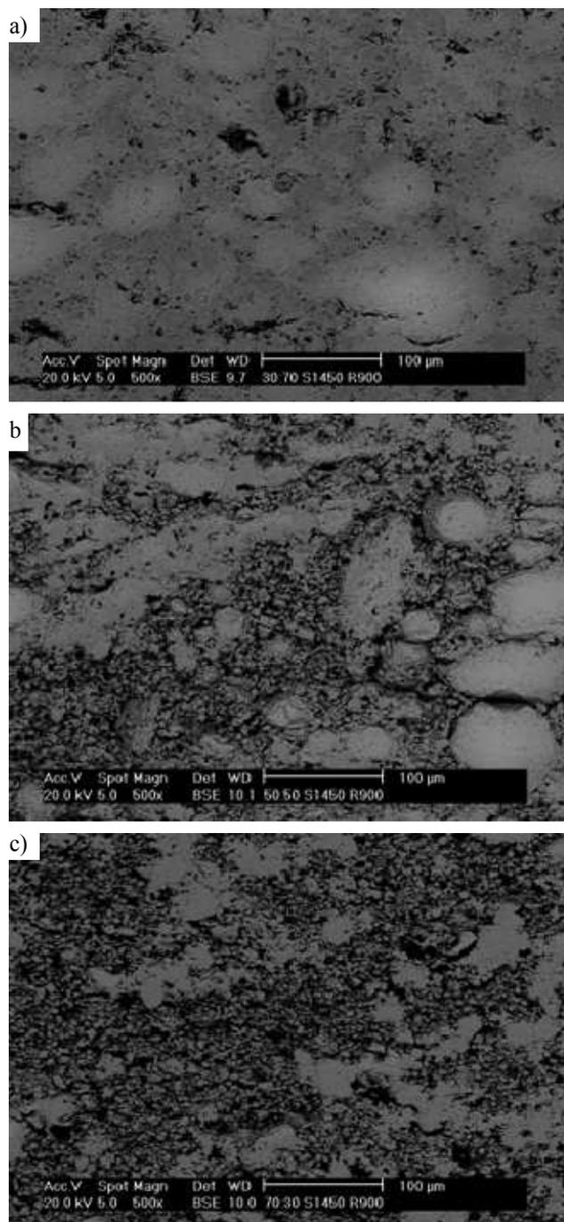
Fig. 6. Structure of samples sintered at 1450°C and reduced at 900°C a)30%, b)50% and c)70% of NiO
