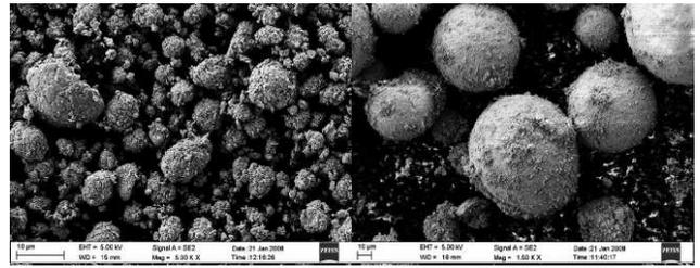
Fig. 1. SEM micrographs of (a) NiO and (b) YSZ powders
