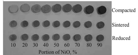
Fig. 2. Investigated samples in compacted, sintered and reduced state
