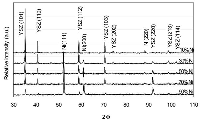
Fig. 4. XRD patterns of reduced samples (at  $800^\circ C$ ) with different amount of YSZ
