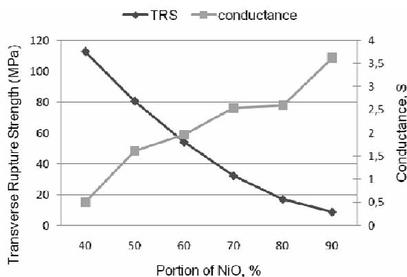
Fig. 8. Mechanical and electrical properties versus volume fraction of NiO
