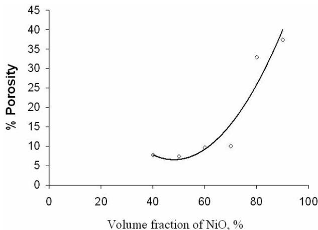
Fig. 7. Open porosity as a function of volume fraction of NiO
