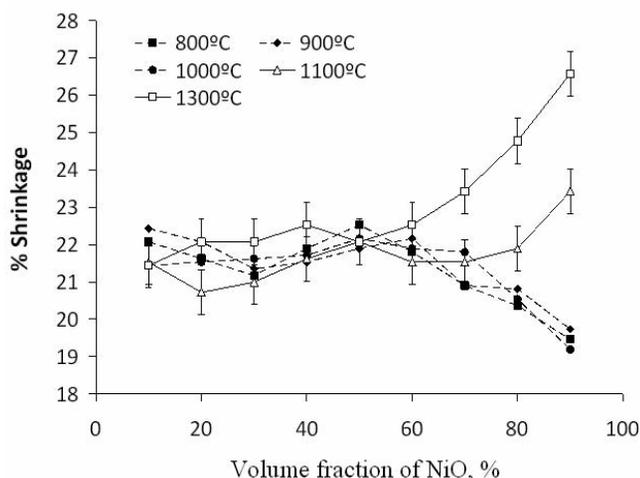
Fig. 5. Shrinkage in relation to reducing temperature for samples sintered at 1400°C with different volume fraction of NiO.
