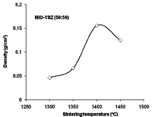
Fig. 3. Sintering curve of 50/50% in vol. NiO-YSZ composite
